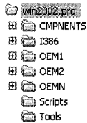
Figure 7-4 For Windows XP Tablet PC Edition, copy the CMPONENTS folder to the root of the distribution folder, side by side with the I386 folder.
