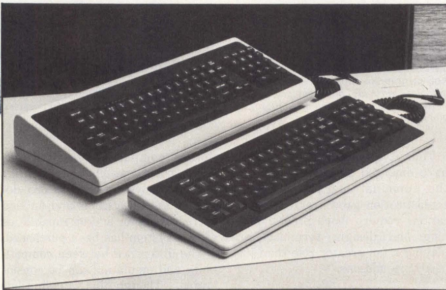
The DEC VT100-like keyboard (right) provides one aspect of thorough terminal emulation. Terminals designed to replace popular terminals such as the VT100 often duplicate the original down to the color of the plastic to ease a user's transition.
