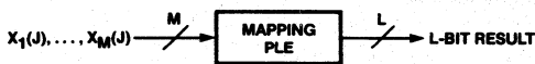
Figure 1. Mapping the j^{\text{th}} Bit from Each of the x_i 's to An L-bit Result
