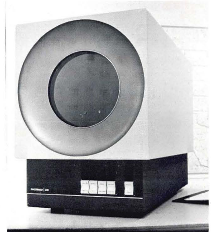
The Dicomed 30 — a direct-view CRT Image Display for high-resolution pictorial information.
