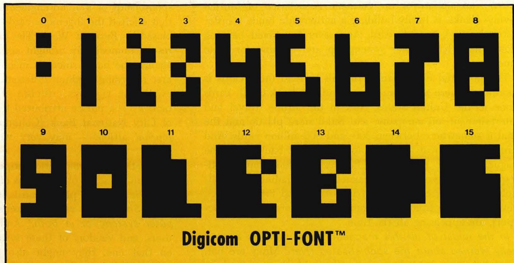
Fig. 1 — This set of sixteen special numeric characters, whose coverage (or apparent grayness) increases with value, is the key to Digicom's direct digital graphics technique.
