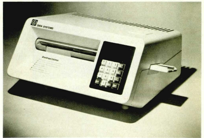
Addressograph-Multigraph's AMCAT terminal — a mag stripe reader.
