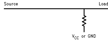
FIGURE 35b. Parallel Termination
