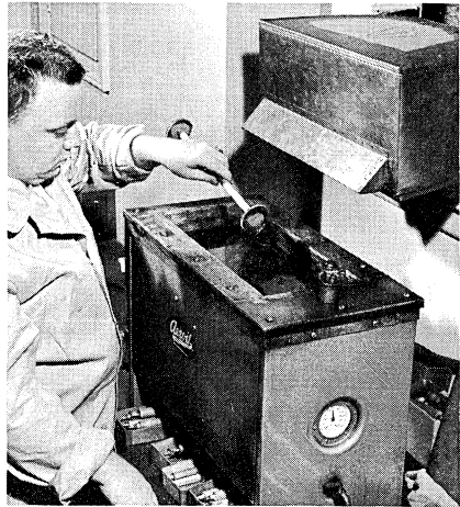
Precision Gear Teeth Being Dipped and Protected to Eliminate Possible Damage During Shipping
