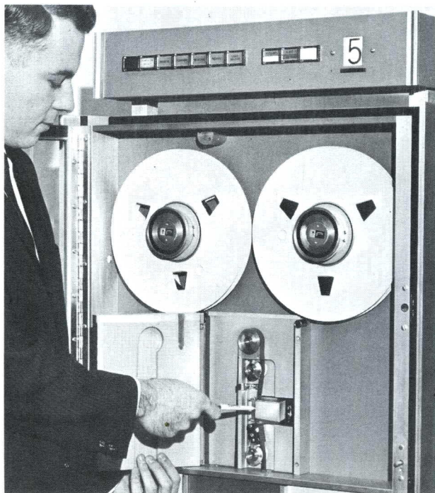
Figure 5. Automatic Tape Loading
