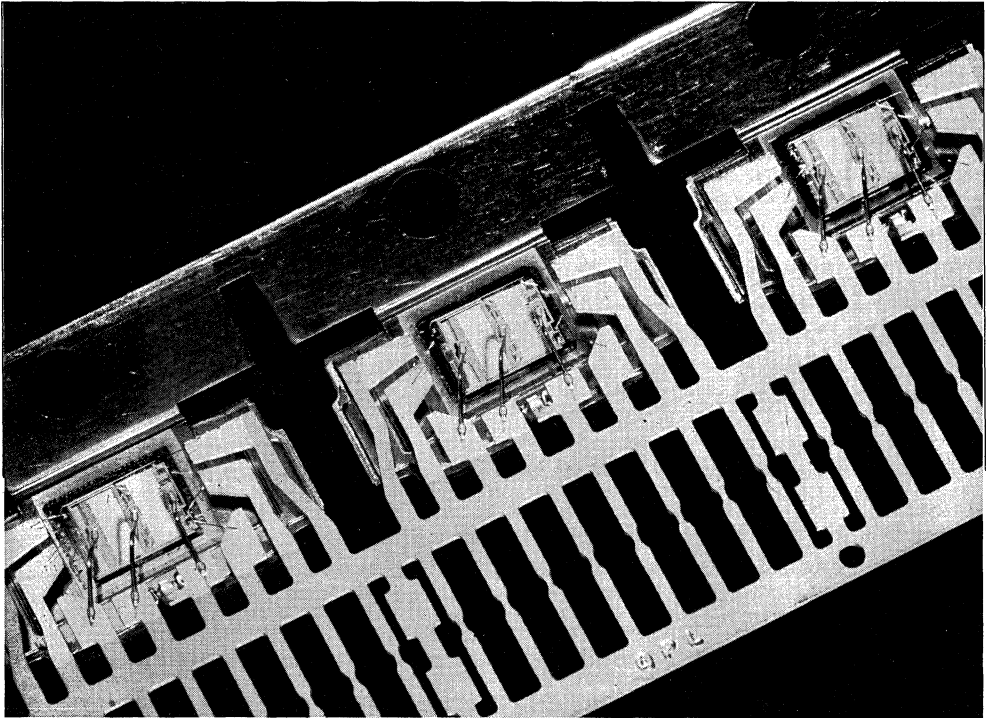
Figure 9: An example of a power IC using mixed wire bonding.
