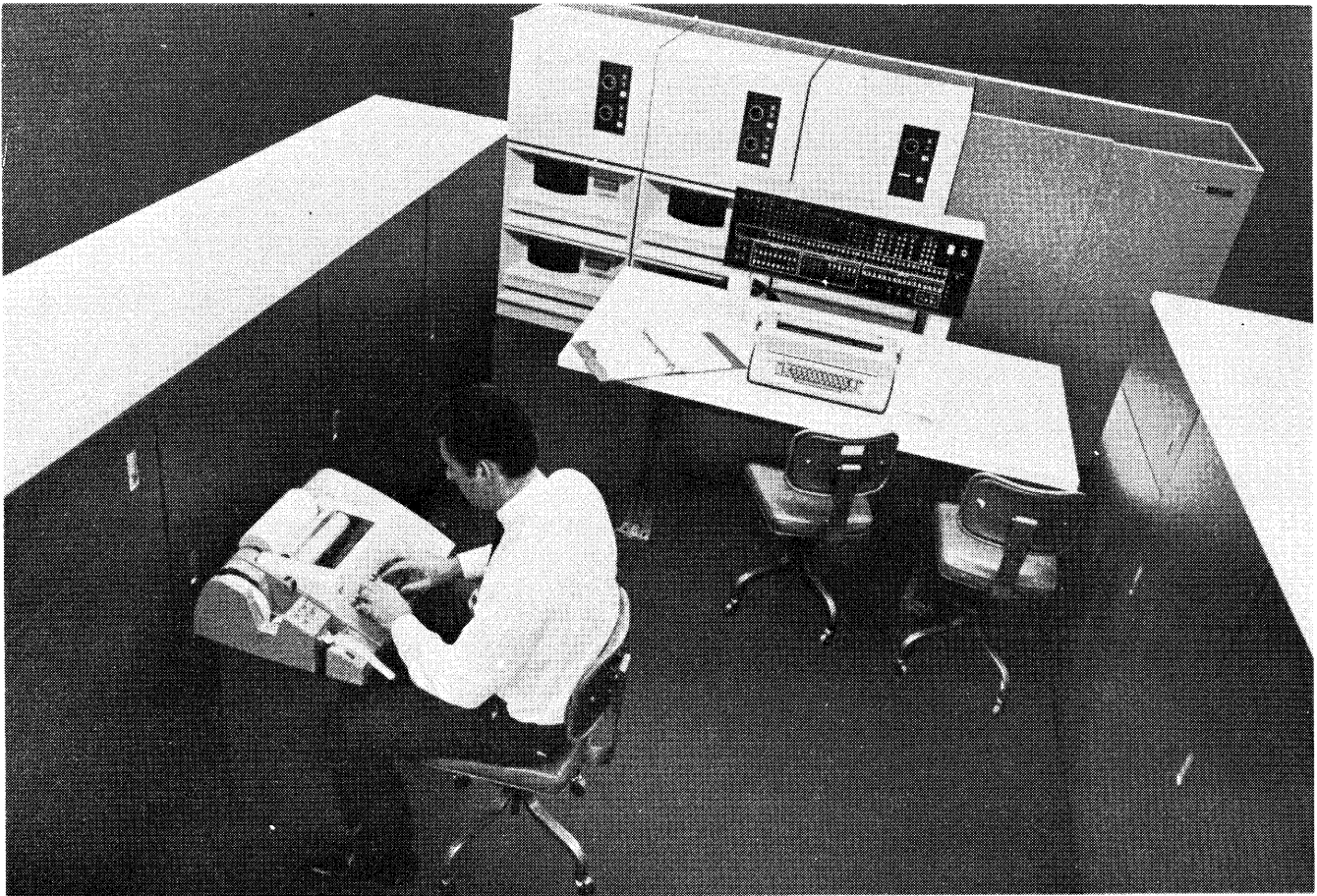
Figure 2. Arithmetic and Language Processor (left), Desk Console and Disk Storage Drive (center), and Supervisory Processor Unit (right)
