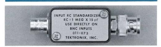
Five input time-constant standardizers are available for standardizing input capacitances of 12 pf, 15 pf, 20 pf, 24 pf, and 47 pf. Each standardizer has an approximate 1 megohm impedance and 2X voltage attenuation.
