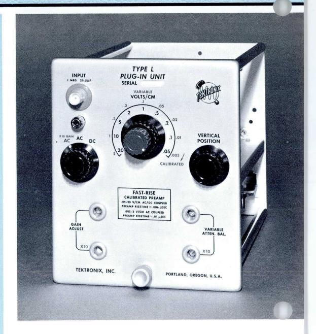
The Type L Fast-Rise High-Gain Unit, duplicates the performance of the Type K and offers increased sensitivity, ac-coupled, to 5 mv/cm. An ac-coupled amplifier increases the sensitivity by a factor of 10 with slightly reduced frequency response and increased risetime. When used with Type 530-Series Oscilloscopes the unit has somewhat reduced frequency response and increased risetime.
