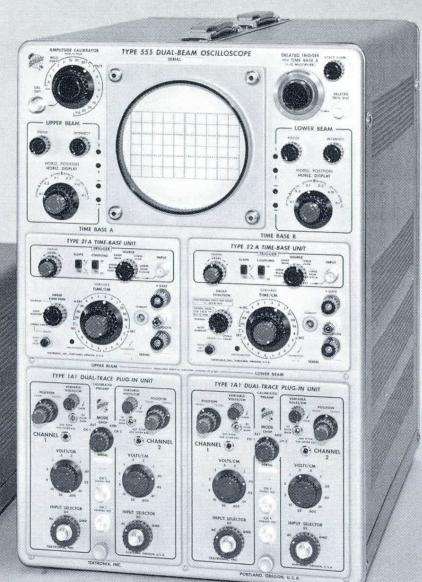
The Type 555 Oscilloscope is a dual-beam laboratory instrument for accurate measurements in the dc to 33 Mc range. Two complete horizontal-deflection systems and two independent vertical amplifiers provide for completely independent deflection of the two beams.
