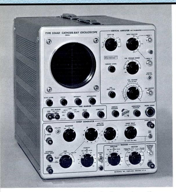
The Tektronix Type 524AD Oscilloscope is a self-contained instrument with the characteristics desirable for maintenance and adjustment of television transmitter and studio equipment. The Type 524AD will prove itself invaluable in enabling the engineer to observe any portion of the television picture — from complete frames to small portions of individual lines.
