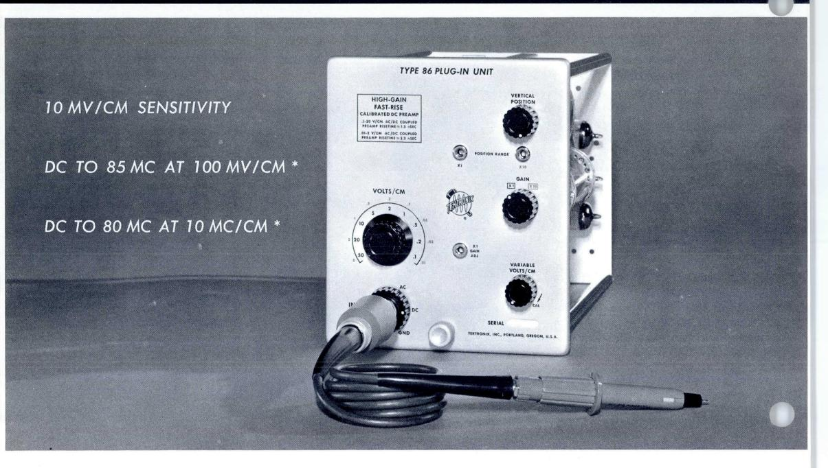
RISETIME of the Type 86 and Type 580-Series Oscilloscope is nominally 4 nsec at 100 mv/cm, always less than 4.2 nsec. At 10 mv/cm, using the 10X Amplifier, risetime is nominally 4.3 nsec, always less than 4.5 nsec. 100 mv/cm 12 db point is at approximately 150 Mc.
