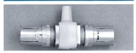
The 50-ohm "T" type pickoff allows signal pickoff from a closed 50-ohm system with minimum disturbance of the system's characteristics. The coaxial "T" incorporates GR Type connectors at each end, with a plastic center collar for probe tip insertions.
