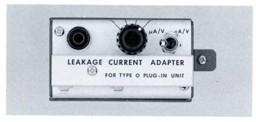
The Leakage Current Adapter, used with the Type O Operational Amplifier Plug-In Unit, adapts the plug-in for measuring the reverse leakage current of semiconductor diodes and small-signal transistors. The adapter may also be used for measuring junction resistance or capacitance.
