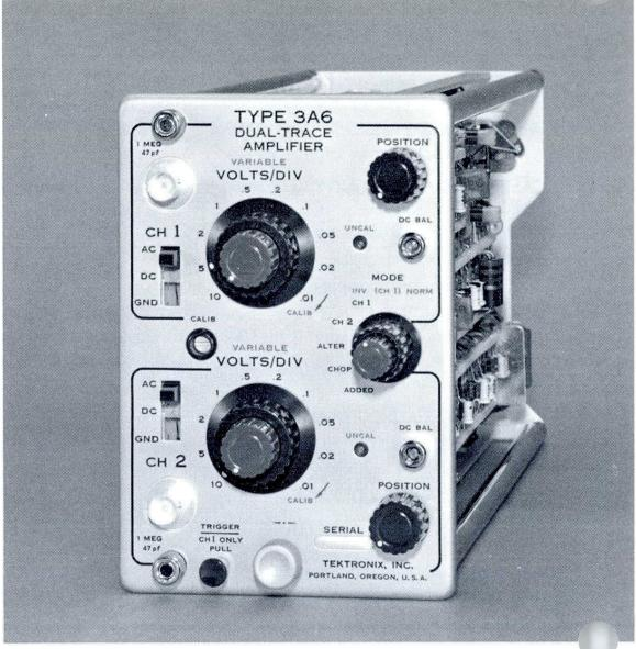
The Type 3A1 and Type 3A6 Amplifiers are general-purpose dual-trace plug-in Units. They are identical in every respect except that the Type 3A1 does not have a signal-delay line. The Type 3A6 does contain an internal 260 nanosecond signal-delay line that allows viewing of the leading edge of the sweep-triggering waveform when using a high-speed time base such as the Type 3B1, 3B3 and 3B4 Time-Base Units\*.
