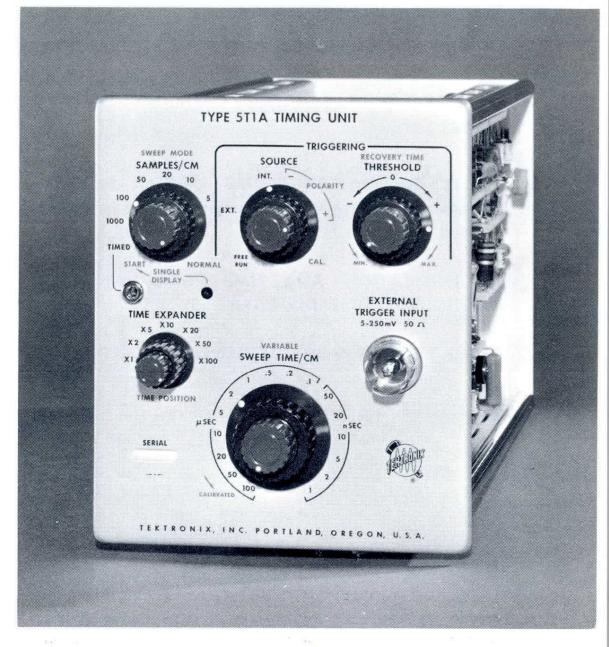
EXTERNAL 50-OHM TRIGGER INPUT is ac coupled (1  $\mu$ sec time constant) and allows direct connection of the Type 5T1A to the trigger signal. Sensitivity is 5 mv for a fast-rise 2-nsec wide pulse. An isolation stage reduces kickout to 5 mv or less, with less than 1/2 nsec decay time constant.
