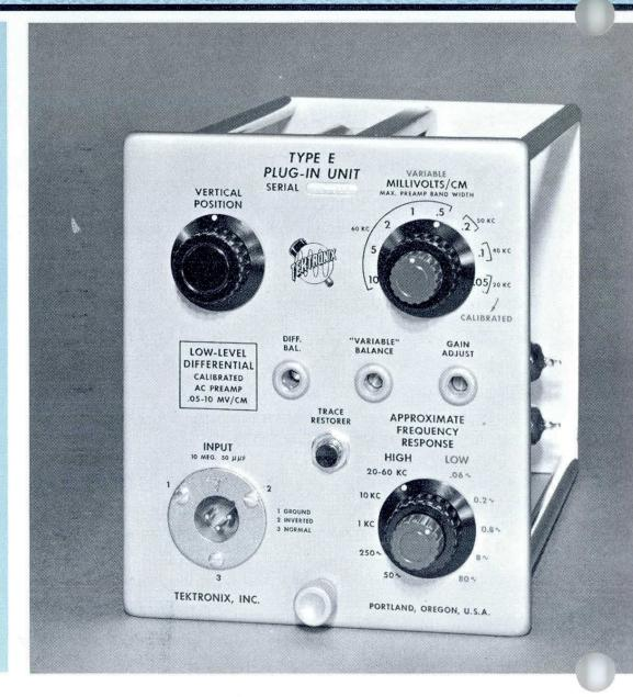
Bandwidth Control—A five-position switch provides for approximate high-frequency 3-db points of 60, 10, and 1 kc; 250 and 50 cycles. Another five-position switch selects the approximate low-frequency 3-db points of 0.06, 0.2, 0.8, 8 and 80 cycles. Restricting the bandwidth to the requirements of the particular application will provide an increase in the signal-to-noise ratio. Input to grids is dc-coupled to provide good rejection at low frequencies.
