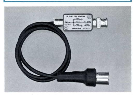
The Adapter is basically intended for use with the Type N Plug-In Unit, but can be used with any Tektronix sampling system except those incorporating the Type RM561 and Type 567 Oscilloscopes. The Adapter converts a 50-volt output from the oscilloscope calibrator to 40 mv at an impedance of 50 ohms for use in calibrating the gain of the sampling system.
