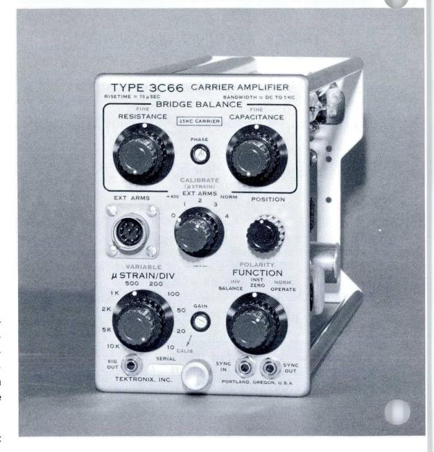
CALIBRATED SENSITIVITY is from 10 microstrain/div (microinches per inch/div) to 10,000 microstrain/div when the Type 3C66 is used with a single strain gage having a gage factor of approximately 2. Uncalibrated continuous control from 10 microstrain/div to 25,000 microstrain/div.
