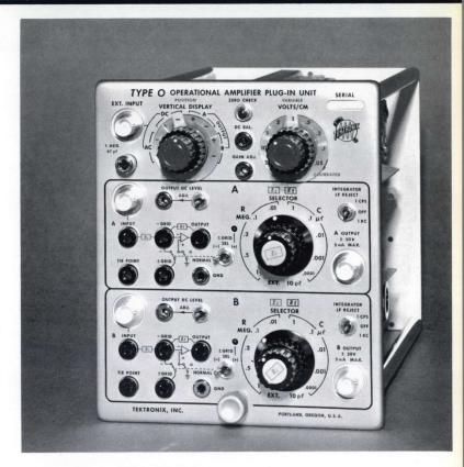
OUTPUT RANGE is  $\pm 50 \text{ V}$ ,  $\pm 5 \text{ mA}$ .
