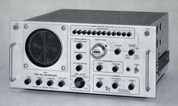
DIFFERENTIAL PHASE MEASUREMENTS-To 0.1°.
