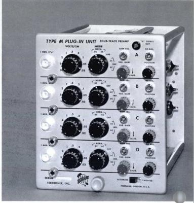
CHANNEL A SIGNAL available at front panel can be connected to oscilloscope external trigger input for stable triggering in the Chopped or Alternate Mode—enabling display of all input signals in true time or phase relationship.
