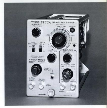
CALIBRATED SWEEP TIME/DIV is from 0.2 ns/div to 10  $\mu$ s/div in 15 calibrated steps, 1-2-5 sequence. Accuracy is within 3%. A variable control permits continuous adjustment uncalibrated between calibrated ranges.
