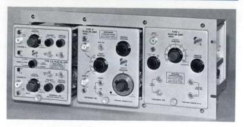
PLUG-IN PREAMPLIFIER STORAGE CABINET mounts in standard rack, available in two types:
