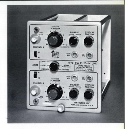
**OPERATING MODES** are: Channel A only; Channel B only; Electronic switching at 100-kHz rate (chopped); Electronic switching on alternate sweeps; Both channels added algebraically  $(\pm A \pm B)$ .
