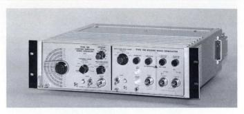
The Rack Adapter converts the latest series of Tektronix Generators for rack mounting. Any combination of two instruments can be mounted side-by-side in 19" rack, occupying only  $5^{1}/_{4}$ " of vertical rack space. Mounting brackets located on the rear of the unit are adjustable for installation in racks of different depths. The brackets can be adjusted for a depth of  $8^{1}/_{2}$ " to  $26^{\prime\prime\prime}$ .
