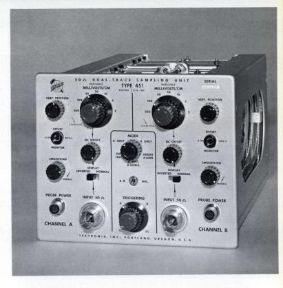
SMOOTHING CONTROL reduces system time jitter and amplitude noises, if needed, when there is sufficient dot density.
