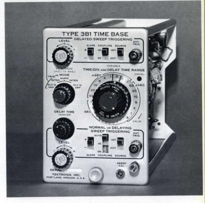
The delayed-sweep generator operates as the display time base in (1) the DELAYED SWEEP position—displaying the portion of the trace which was intensified in the INTENSIFIED position . . . with time-jitter less than 1 part in 20,000 of the maximum available delay interval—and (2) the jitter-free TRIGGERED, DELAYED SWEEP position—displaying the portion of the trace which was intensified in the TRIGGERED, INTENSIFIED position.
