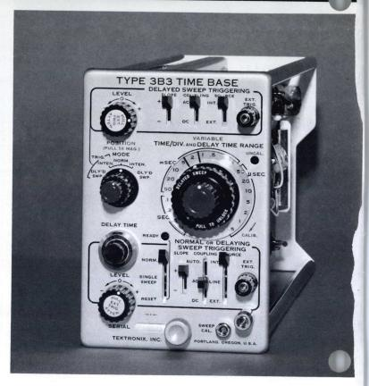
The delayed-sweep generator operates as the display time base in (1) the DELAYED SWEEP position—displaying the portion of the trace which was intensified in the INTENSIFIED position...with time-jitter less than 1 part in 20,000 of the maximum available delay interval—and (2) the jitter-free TRIGGERED, DELAYED SWEEP position—displaying the portion of the trace which was intensified in the TRIGGERED, INTENSIFIED position.
