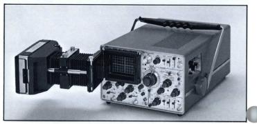
The Type 453 with the Tektronix C-30 Camera.
