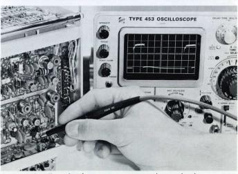
Small probe for easy access to dense circuitry.
