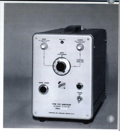
The Type 1121 Wide-Band Amplifier is a cascaded-input, low-noise amplifier designed with Tektronix precision, quality, and style. It increases the amplitude of low-level wideband signals; thus increases the sensitivity of the oscilloscope or other associated instrument with which it is operated.
