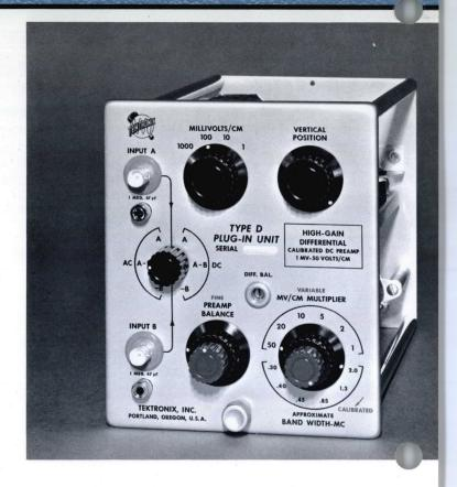
STABILITY is from 2 to 5 mV/h (normal drift).
