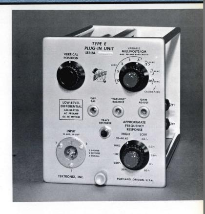
COMBINED NOISE AND HUM is 5 µV, RMS (maximum) with input grids grounded at the input connector.
