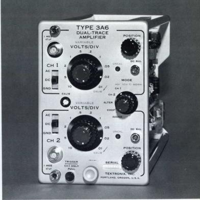
The Type 3A1 and Type 3A6 Amplifiers are general-purpose dual-trace plug-in units. Performance of the two units is the same except that the Type 3A1 does not have a signal-delay line. The Type 3A6 does contain an internal 260-nanosecond signal-delay line that allows viewing of the leading edge of the sweep-triggering waveform when using a high-speed time base such as the Type 3B1, 3B3, 3B4, and 3B5 Time-Base Units.\*
