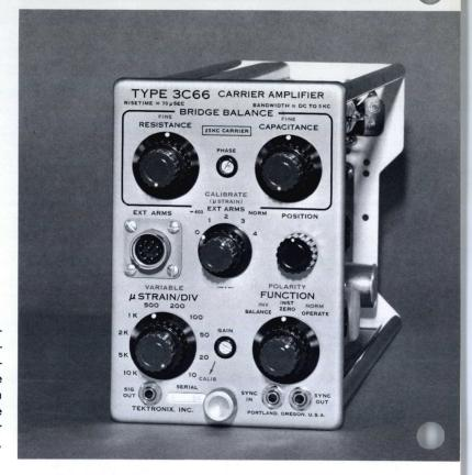
CALIBRATED DEFLECTION FACTOR is from 10 microstrain/div (micro-inches per inch/div) to 10,000 microstrain/div when the Type 3C66 is used with a single strain gage having a gage factor of approximately 2. Uncalibrated continuous control from 10 microstrain/div to 25,000 microstrain/div.
