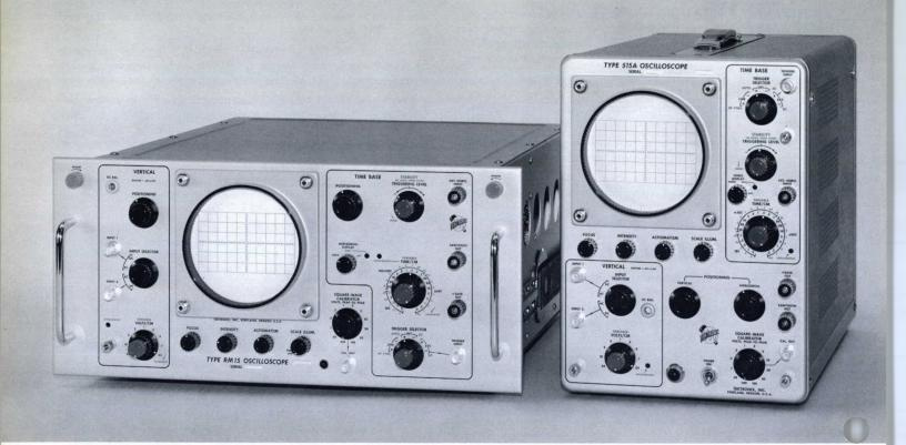
The Tektronix Type 515A is a DC-coupled general-purpose cathode-ray oscilloscope combining reliable Tektronix oscilloscope circuitry in a compact instrument. Wide sweep range of 0.04  $\mu s/cm$  to 6 s/cm, DC to 15 MHz bandwidth, and calibrated deflection factor to 0.05 V/cm qualify the Type 515A for general-purpose laboratory work and for many field applications.
