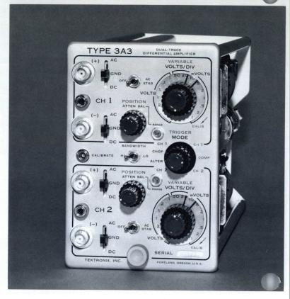
DISPLAY MODES include CH 1, CH 2, or dual-trace with either chopped or alternate switching. In chopped operation, electronic switching occurs at approx a 250-kHz rate to show successive  $2-\mu s$  segments of each trace. Chopped transient blanking is provided.
