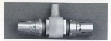
The 50-ohm "T" type pickoff allows signal pickoff from a closed 50-ohm system with minimum disturbance of the system's characteristics. The coaxial "T" incorporates GR Type connectors at each end, with a plastic center collar for probe tip insertions.
