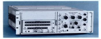
For rackmounting most Tektronix generators in a standard 19-inch wide rack. The rack height is 51/4 inches, rack depth is 193/4 inches. Rack adapter includes slide-out assemblies. Shipping weight is approx 24 lb.
