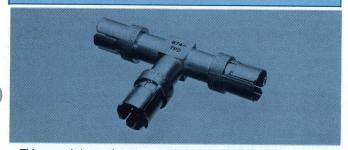
This coaxial tee has a 16.67-ohm resistor in each leg, connected so that the tee looks like 50 ohm if two legs are terminated in 50 ohm. It is designed for use in broad-band  $50-\Omega$  systems where the mismatch introduced by ordinary "Tee" connectors is undesirable. It is especially useful in a time-domain reflectometer set-up where test line, pulser, and oscilloscope must be coupled with a minimum of reflection-producing discontinuities.
