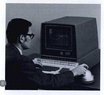
The most common usage of time-sharing terminals today is calculation. With FORTRAN, engineers and scientists can create complex and highly repetitive routines for the computer to handle, insert the variables or parameters, and in a very short time obtain output. This allows exploration of a broad range of possible solutions, and decision-making based on analysis of a large sample or of ALL possible outcomes.
