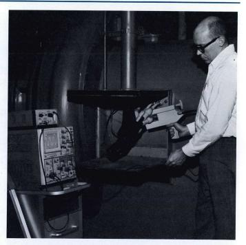
Typical application of CT-5 clip-on High Current Transformer, P6042 DC Current Probe and 7504 Oscilloscope measuring the running current of a 1500 hp delta-connected induction motor.
