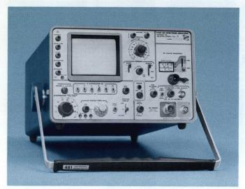
The Type 491 MOD 139M has a center frequency range of 1.5 GHz to 40 GHz with optional accessories. The chart on the first page defines the Frequency Range and Minimum CW Sensitivity (S + N = 2N). The appearance is the same as that of the Type 491 with the following exceptions: the A and B band inputs are removed and the center frequency range dial is hanged to reflect the reduction in the number of frequency ands.
