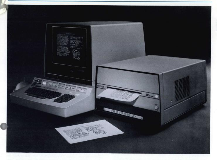
The T4002 Graphic Computer Terminal shown above with the 4601 Hard Copy Unit.
