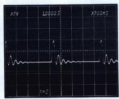
Fig 2: Output of 7D14 trigger circuit is added to the displayed signal. This allows the user to determine which signal is being counted.
