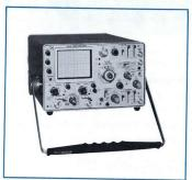
453A Oscilloscope—The portable 453A is a dual-trace 60-MHz oscilloscope with deflection factors to 5 mV/div, sweep rates to 5 ns/div and delaying sweep. A CRT with 8 x 10 divisions (0.8 cm/div) and 14-kV accelerating potential provides a bright, high-resolution display for field maintenance as well as laboratory applications.
