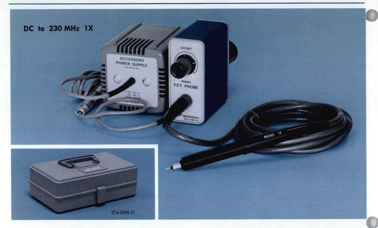
The P6045 FET Probe offers capabilities for measuring small, high-frequency signals. Unlike many general-purpose probes which require built-in attenuation to reduce circuit loading, the P6045 utilizes a field effect transistor, resulting in reduced loading without sacrificing the gain of the measurement system.
