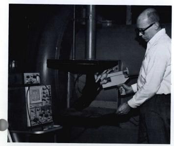
Typical application of CT-5 clip-on High Current Transformer, P6042 DC Current Probe and 7504 Oscilloscope measuring the running current of a 1500 hp delta-connected induction motor.
