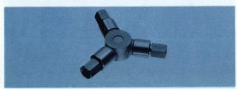
This coaxial tee is designed for use in broad-band,  $50-\Omega$  systems where the mismatch introduced by ordinary "Tee" connectors is undesirable. Load isolation is nominally 6 dB while the voltage attenuation ratio is nominally 2X (input to either load arm, other load arm terminated in a standard  $50-\Omega$  termination). Maximum VSWR is 1.50 from DC to 12.00 GHz and 1.90 from 12.01 to 18.00 GHz.
