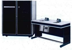
The S-3150 is a high-speed, disc-programmed, dynamic, functional and DC-test system for integrated circuits. The S-3150 includes a small computer (D.E.C. PDP-8L) for data acquisition and program writing.
