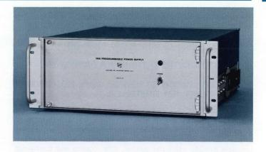
Programmed Compliance Voltage Limit Range-Plus current, 0 to  $+70 \,\mathrm{V}$  in  $5 \,\mathrm{V}$  increments. All 4 bits programmed gives +100 V. Minus current, 0 to -70 V in 5 V increments. All 4 bits programmed gives -100 V.
