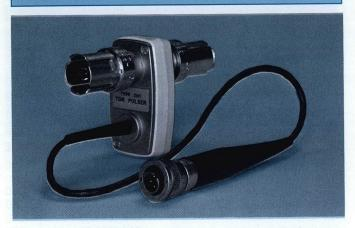
The Type 281 Time-Domain Reflectometer Pulser is designed for use with Tektronix Type 1S1 and 3S1 Sampling Plug-Ins. It converts these general-purpose sampling plug-ins to an easy-to-use TDR system. Power is obtained from their probe power connector.
