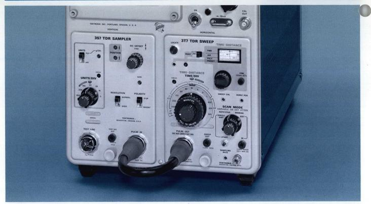
curate within 1%. The TIME-DISTANCE MULTIPLIER provides positions of X0.1, X1, and X10 the tape dial reading. Optional tape dial (see below) is calibrated in metric units.
