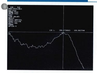
The above photograph pictures the clearly visible parallax-free, crosshair cursor generated by the 4901 or 4902. The cursor always covers the entire X, Y dimensions of the display. Positioning accuracy is within one LSB along each axis.
