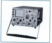
provide the performance to solve difficult measurement problems such as resolving pulses with low-nanosecond periods.
