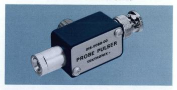
The tunnel-diode pulser is used to adjust the P6045 FET Probe for optimum response. The pulser is designed to be driven by the 100-V output of the oscilloscope calibrator. Risetime of the probe pulser is less than 0.5 ns.
