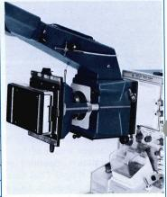
Camera mounted to 576 Curve Tracer using adapter frame and standard 5-inch round CRT adapter. Corrector lens is gray piece in middle of camera.
