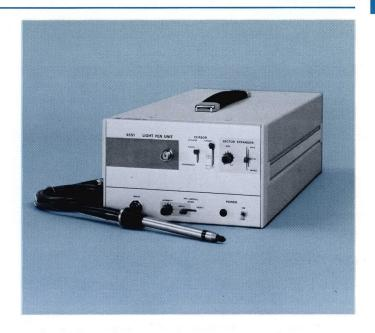
as the gap is bridged and the pen is held against the display, the cursor tracks the pen movements. To stop the cursor movement, the operator simply lifts his finger.
