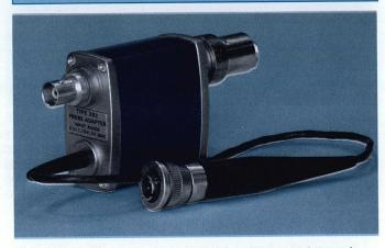
The Type 282 permits the use of conventional high-impedance probes with  $50-\Omega$  sampling plug-in units, such as Types 1S1 and 3S1. Power is obtained from their probe power connector. The Type 282 Mod 125D is a similar unit for use with the Types S-1 and S-2 in Type 3S2, 3S5 and 7S11 sampling plug-ins. Power is obtained from the accessory power supply.
