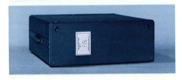
The Tektronix Type 113 Delay Cable has a delay of 60 ns and a characteristic impedance of  $50\,\Omega$ . In general it is used in those sampling applications where the vertical amplifier does not contain internal delay lines and the triggering of the sweep is external and signal delay is required.
