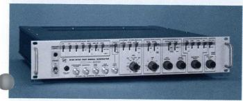
The 144 NTSC Signal Generator is a compact, solid-state source of high-quality color television test, sync, and burst signals for 525-line, 60-Hz field, cable, and broadcast TV systems. Combined in one compact unit are the signals needed to accurately test, evaluate, and adjust CATV, laboratory, and standard broadcast color video equipment.
