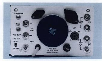
Rear panel of Type 528 Waveform Monitor.
