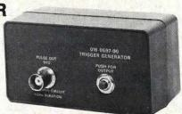
The Manual (one shot) Trigger Generator is a self-contained, battery-operated, handheld device for manually generating a single pulse. This adapter is used to start a pulse, ramp, sweep, or complete sequence of events on instruments which do not have a manual trigger button or where a remote operation capability is desired, such as some oscilloscopes and the PG 501, PG 505, and RG 501.
