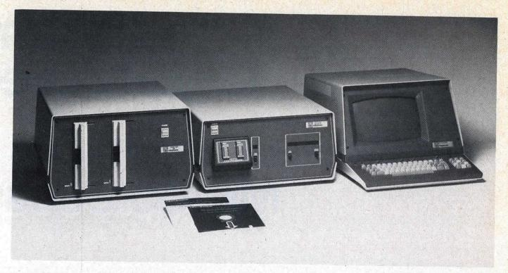
The 8002A Microprocessor Lab consists of the 8002A Mainframe with 32K of Program Memory, and the dual flexible disc unit. Recommended optional peripherals are the CT 8100 Crt Terminal, the CT 8101 TTY Terminal, the 4024/4025 Computer Display Terminals, or the LP 8200 Line Printer.
