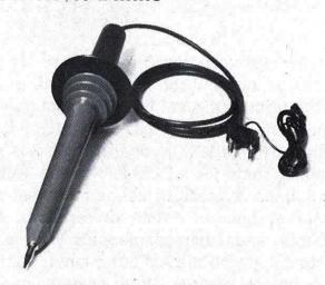
The High Voltage Probe will measure dc voltages from 1 kV to 40,000 volts with an accuracy of 1% at 25,000 volts. The division ratio is 1000:1. Common uses include measuring anode voltages on monitors or oscilloscopes.
