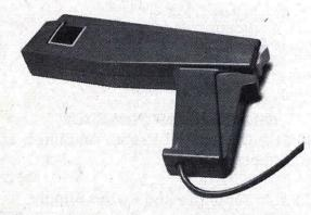
100A Ac and Dc Current Measurements Dc to 15-MHz Bandwidth Peak Pulse Measurements to 500 A Ac or Dc Coupling 1 inch x 0.830 in Jaw Opening Minimal Loading—0.02  $\Omega$  Insertion Z at 1 MHz, 0.15  $\Omega$  at 15 MHz
