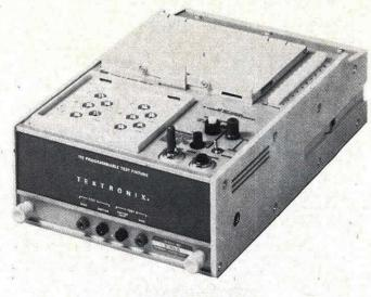
The 172 Programmable Test Fixture, when used with the TEKTRONIX 576 Curve Tracer, permits the operator to program a sequence of tests of J FET's, transistors, and diodes.
