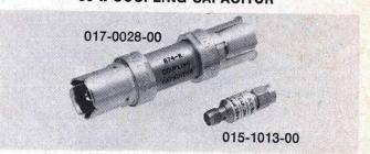
The coupling capacitor is a short length of coaxial line having a disc capacitor (4700 pF,  $\pm 20\%$ ) in series with the inner conductor. Reflection ratio (in 150 ps tdr system), max is 0.03. Voltage rating is 200 V.
