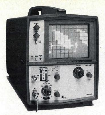
T921 15 MHz Single-Trace Oscilloscope
