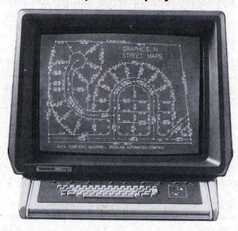
25" Graphics Display for more Information Capacity Detachable Keyboard and Display Local Digitizing Capabilities PLOT 10 Compatible
