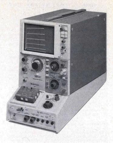
The 577 Curve Tracer System, when used with the 177 Standard Test Fixture, is a smaller and lighter configuration that retains many of the important features and performance of the 576. The 577 also accepts the 178 Linear IC Test Fixture. The major features that separate the 577 from the 576 are storage and the emphasis on low current measurements.
