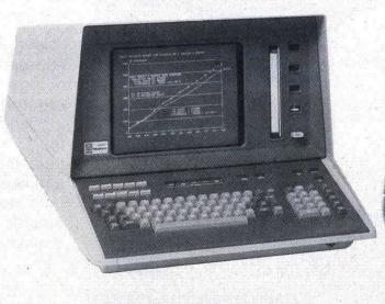
The 4907 File Manager offers many features available only on large computer systems. A real-time clock providing date and time of file activities, up to 9 simultaneously open files, file security (passwording and execute only) and dynamic allocation of file space are examples of these enhancements. No bootstrapping of system software is ever required. An advanced multiple level file-
