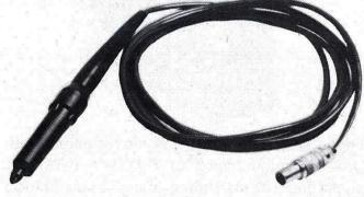
The P6430 Temperature Probe is used with the DM 502 for sensing temperature from  $-55^{\circ}\text{C}$  to  $+150^{\circ}\text{C}$ . The temperature sensing element consists of a transistor and is installed in the probe's nose tip. Temperature is measured by applying the flat surface of the probe's tip to the device being measured. The probe can be immersed vertically, approximately two inches in a liquid, for temperature sensing and still retain water tightness.
