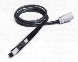
20A Ac and Dc Current Measurements Dc to 50 MHz Bandwidth Peak Pulse Measurements to 50A, 50,000A with the CT-5 Current Probe Clip-on Probe Ac or Dc Coupling Small Loading—0.1  $\Omega$  Insertion Z at 5 MHz,  $0.5~\Omega$  at 50~MHz
