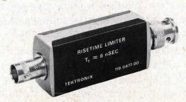
For use with the PG 502 Pulse Generator which has a pulse rise and fall time of less than one nanosecond. In some applications, such as TTL logic where slower rise time is needed, this fast pulse can be limited to six nanoseconds by using the rise time limiter.
