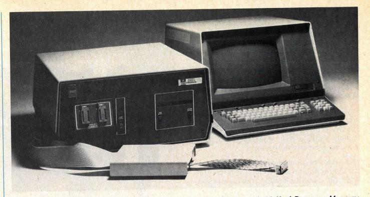
The 8001 Microprocessor Lab consists of the 8001 Mainframe with 16 K of Program Memory. Microprocessor Support Packages for microprocessors are optional. A Microprocessor Support Package includes an emulator ROM, an emulator processor, and a prototype control probe. The CT 8100 Crt Terminal, CT 8101 TTY Terminal, 4024/4025 Computer Display Terminals, or the LP8200 Line Printer are recommended optional peripherals.
