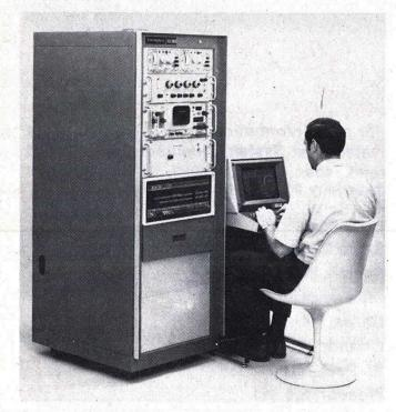
The S-3003 is a computer-controlled waveform digitizer, which can be a stand-alone test system by using either a Tektronix controller or your computer, or can be interfaced to your test system as an ac measurement sub-system. The S-3003 includes the R568 Readout Oscilloscope, the 3S6 and 3T6 Plug-in Units, and the 1340 Data Coupler, which is comprised of interface circuit cards for the R568 scope, the Waveform Digitizer and optional interfaces to your computer.
