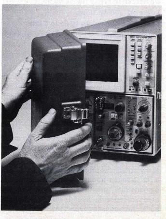
Option 08 protective front cover is shown on 7613 Mainframe.
