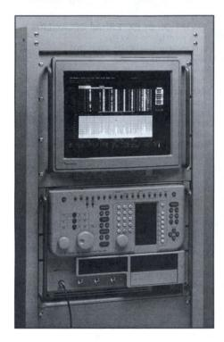
3052 Digital Spectrum Analyzer System
