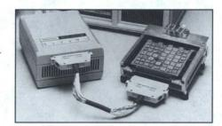
The MIL-STD 1750A emulator supports the unique requirements for integrating software into the target environment. The emulation system can be used to test software written in assembly, or in a high-order language such as Ada, JOVIAL, or CMS-II. A series of probe adapters are available for connection into the various processor environments. These probe adapters can be used to connect the emulator to a board, a bus, or to the CPU's mechanical enclosure.
