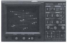
WFM-300 Component Television Waveform Monitor with Vector Display.
