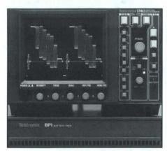
1740 Waveform/Vector Monitors with optional carrying case and battery pack.
