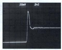
Circuit faults such as high-frequency pulse overshoot and ringing can easily be observed with the 7104/R7103's 1-GHz bandwidth.
