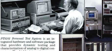
characterization of analog to digital converters. The highly interactive mouse-based interface allows fast parameter changes and instantly displays results in color graphics on a windowed display. The system is easily expanded when more
