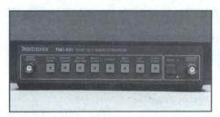
TSG-100 Test Signal Generator.
