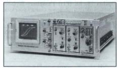
The R7103 requires only seven inches of rack height in a standard 19-inch rack. It is fancooled and comes complete with slideout
