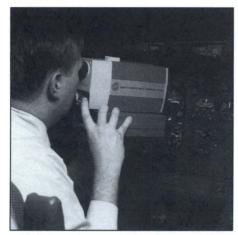
Measuring Luminance with the Tektronix J16/J6523.
