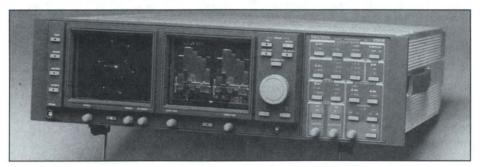
Portability kit provides feet, tilt stand, carrying handle, and (not shown) front and rear covers.
