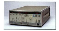
High Resolution, Accuracy, and Speed Ten-bit vertical resolution digitizer (rates up to 200 megasamples per second with long record lengths), the RTD710A provides excellent resolution of fine signal details. See page 443.
