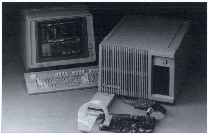
The DAS 9220 mainframe and the color display form the cornerstone of the 9200 Series.
