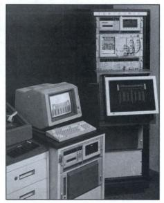
Options for rack conversion, rear-to-front signal routing, and DMA transfer of waveform data and measurement results make the 11401/11402 ideal for systems applications.
