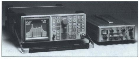
2710 Spectrum Analyzer and the 1405 TV Sideband Adapter.
