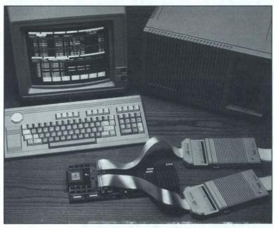
Disk-based mnemonics and single-connection probe adapters make DAS 9200 microprocessor support versatile and easy to use. Refer to page 320.
