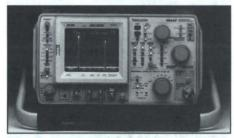
494AP 10 kHz to 325 GHz Spectrum Analyzer
