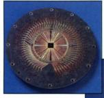
Very High Density Probe Card for VLSI Testing
