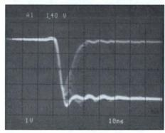
The metastability in this high-repetition rate flip-flop output occurs only once in a million normal cycles, yet is clearly visible, thanks to the MCP's high visual writing speed.
