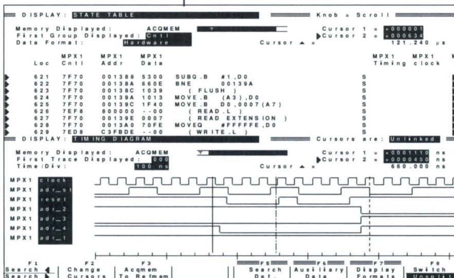
PRISM's split screen display can display both state and timing at the same time. The "link cursor" option links the two displays together so as one display scrolls, the second display stays in sync.
