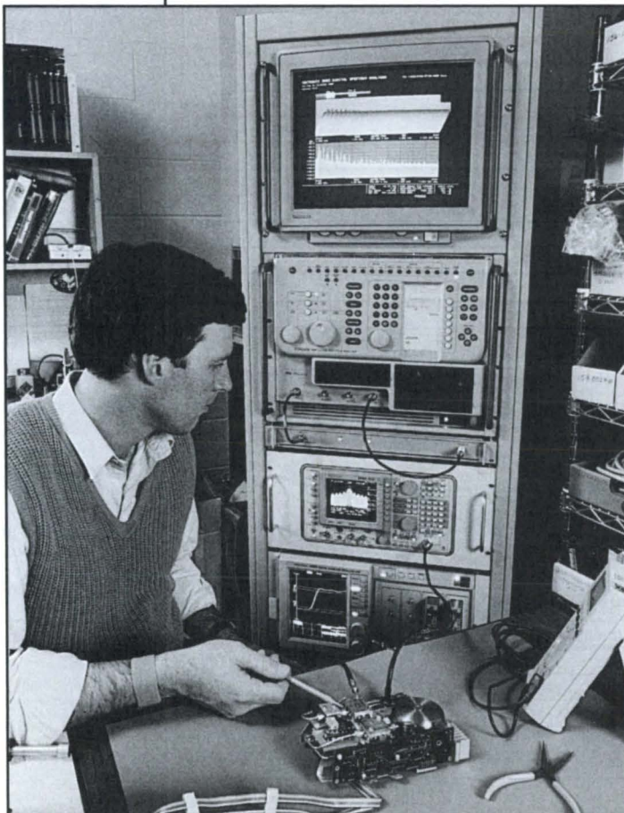
The RF160 Down Converter depicted in a measurement system. In this case a microwave carrier signal is applied to a Tektronix 2782 Spectrum Analyzer. The IF output of the analyzer is then down converted by the RF160, effectively extending the analysis range of the 3052.
