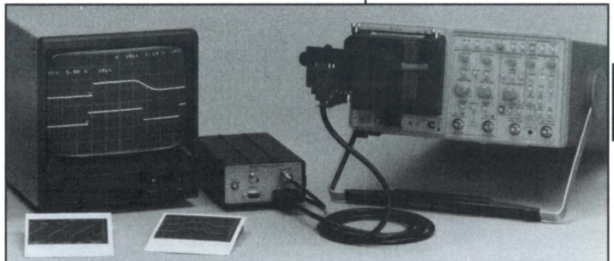
C1002 Video camera, HC02 video copier documenting a 2467B oscilloscope's display using a DX02 power supply.
