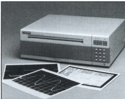
The HC02 can make prints from video, PC CGA graphics, or printer text.
