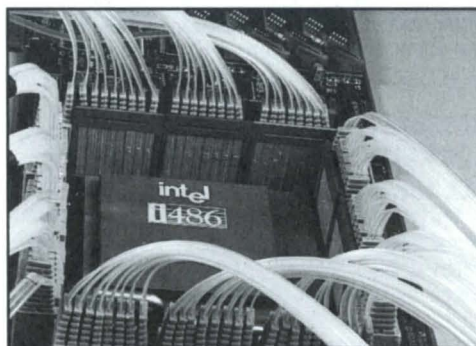
The high-bandwidth probes and advanced 100 MHz clocking state machine of the 92A96 allow the 92A96 to interfaced to virtually any processor or bus without a complex, bulky hardware interface.
