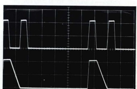
Dual-trace capability makes most measurements easier; pulse circuit analysis is but one application.
