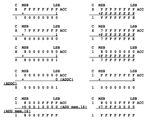
Example 7–12 shows an implementation of two 64-bit numbers added to each other to obtain a 64-bit result.
