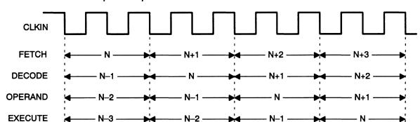
Figure 3-14. Four-Level Pipeline Operation
