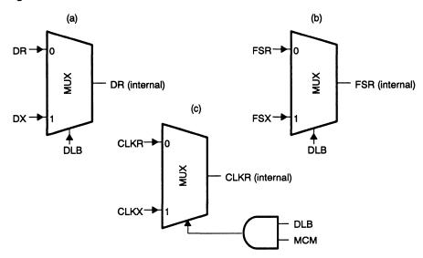
CLKR is driven by CLKX if MCM=1. But if MCM=0 while DLB=1, then CLKR is taken from the CLKR pin. This allows for external clock generation of these signals during digital loopback mode. If DLB=0, then normal operation occurs where DR, FSR, and CLKR are all taken from their respective pins.
