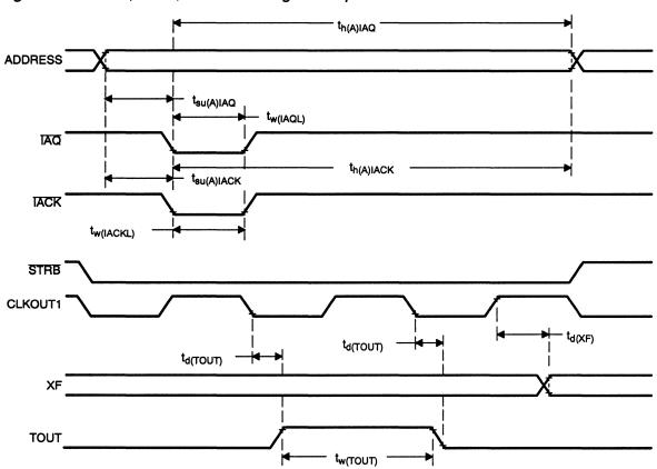
Figure A-13. TAQ, TACK, and XF Timings Example With Two External Wait States
