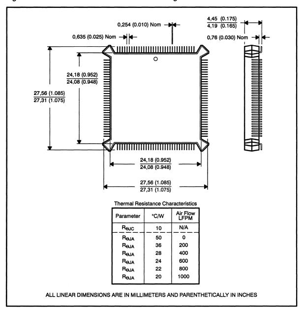
Note: The contact points are within 0,15 (0.006) of being planar.
