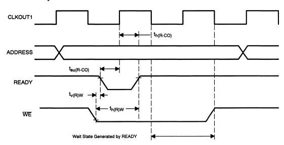
Figure A–11. Ready Timing for Externally Generated Wait States During an External Write Cycle
