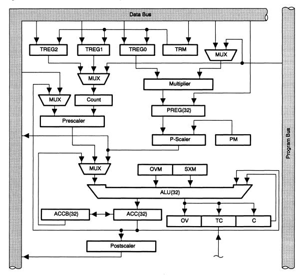
Figure 3-12. Central Arithmetic Logic Unit
