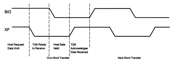
If the 8-bit transfer mode is selected, the lower eight data lines are read from port 50h. The upper byte on the data bus is ignored. The 'C50 reads two 8-bit words to form a 16-bit word. The low byte of a 16-bit word should follow the high byte.
