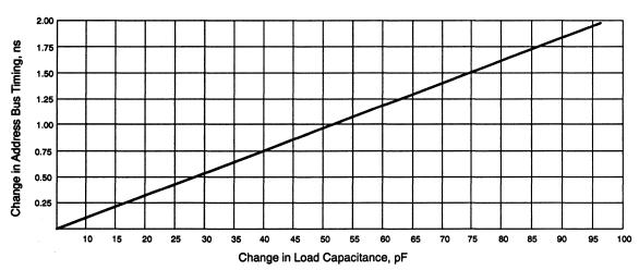
Figure A-9. Address Bus Timing Variation With Load Capacitance
