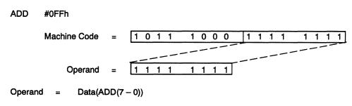
In the case of the long immediate operand, the operand immediately follows the opcode in the program sequence. The long immediate operand is 16 bits long. Figure 3–6 shows an example of long immediate mode. In this example, the second word of the two-word instruction is added to the ACC by the CALU.
