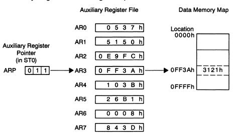
Figure 3-10. Indirect Auxiliary Register Addressing Example
