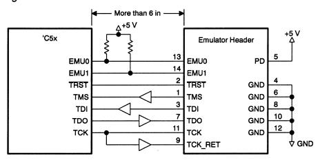
The EMU0 and EMU1 signals must have pullups to 5 volts. The pullup resistor value should be chosen to provide a signal rise time less than 10 μs. A 4.7-kΩ resistor is suggested for most applications. EMU0 – 1 are I/O pins on the 'C4X and 'C5X; however, they are only inputs to the XDS510. In general, these pins are used in multiprocessor systems to provide global run/stop operations.
