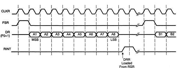
Figure 5-11. Burst-Mode Serial Port Receive Operation
