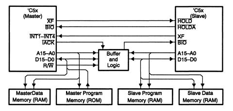
The master 'C5x device takes complete control of the slave's external memory by asserting HOLD low via its external flag (XF). This causes the slave to place its address, data, and control lines in a high-impedance state.
