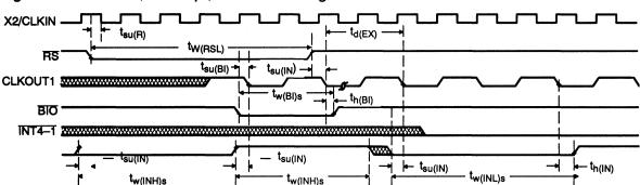
Figure A-12. Reset, Interrupt, and BIO Timings
