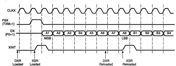
Figure 5-15. Serial Port Transmit Continuous Operation
