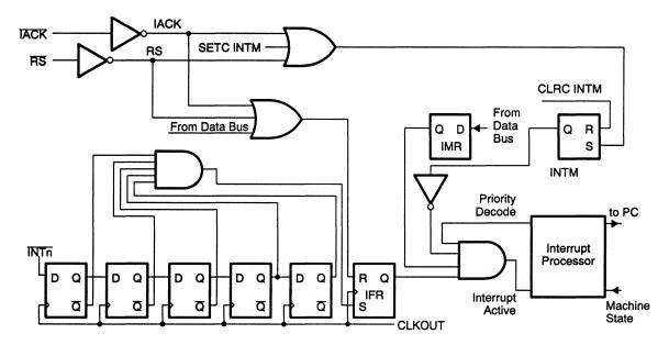
If the INTM bit and mask registers have been properly enabled, the interrupt signal is accepted by the processor. An  $\overline{IACK}$  signal is then generated. The  $\overline{IACK}$  clears the appropriate interrupt edge flip-flop and sets the INTM =1. The logic is the same for  $\overline{INT1}$ – $\overline{INT4}$ .  $\overline{NMI}$  uses the same logic, except that it is not affected by IMR or INTM status.
