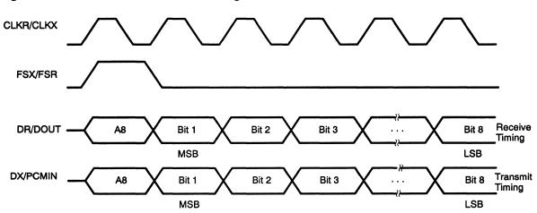
Figure F-5. DSP/Combo Interface Timing
