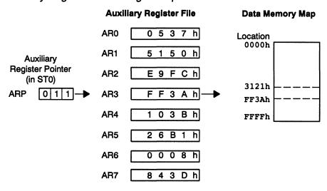
The auxiliary registers and the ARP can be updated directly from data memory, the accumulator, or the product register, or by an immediate operand defined in the instruction. The contents of these registers can also be stored in data memory or used as inputs to the CALU. These registers appear in the memory map as described in Table 6–8.
