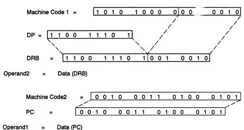
Registered block memory addressing mode operates like the long immediate addressing mode with the exception that the address comes from BMAR. The advantage of this technique is that the address of the block of memory to be acted upon can be changed during execution of the program. The address in long immediate addressing mode resides in the program flow and cannot be easily changed. Figure 3–9 shows an example of registered block memory addressing mode.
