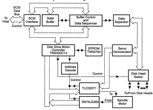
Figure F-9 shows a block diagram of a disk drive control system.
