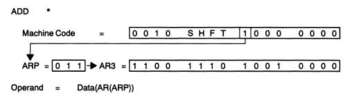
The operand may reside as part of the instruction machine code. In the case of the short immediate operand, the operand is contained in the single-word instruction. These short immediate operands vary in length from 1 bit on the SETC instruction to 13 bits on the MPY instruction. Figure 3–5 shows an example of short immediate mode. Note that, in this example, the lower eight bits are the operand and will be added to the ACC by the CALU.
