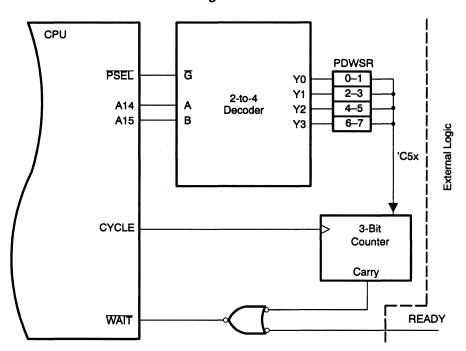
Figure 5-3. Software Wait-State Generator Block Diagram
