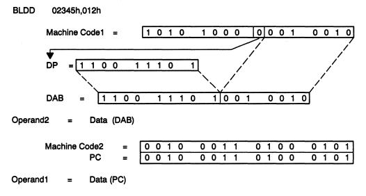
The registered block memory addressing mode operates like the long immediate addressing mode with the exception that the address comes from the BMAR register. The advantage of this technique over long immediate addressing is that it allows the address of the block of memory to be changed in runtime. On the other hand, the address in long immediate addressing mode resides in the program flow and cannot be easily changed. Figure 6–9 shows an example of registered block memory addressing mode.
