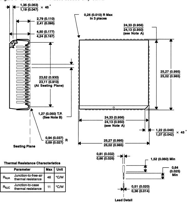
Figure D-2.'C25 68-Pin Plastic Leaded Chip Carrier
