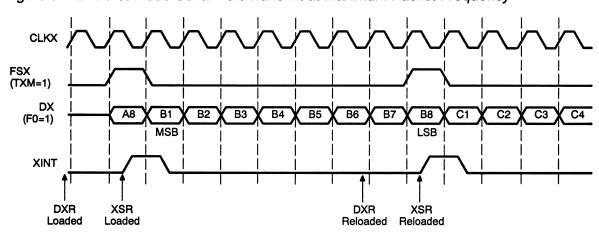
Figure 5-12. Burst-Mode Serial Port Transmit at Maximum Packet Frequency
