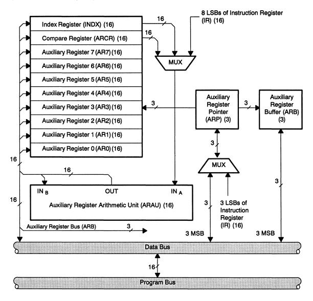
As shown in Figure 6–11, the index register, the compare register, or the eight LSBs of the instruction register can be connected to one of the inputs of the ARAU. The other input is fed by the current AR (being pointed to by ARP). AR(ARP) refers to the contents of the current AR pointed to by ARP. The ARAU performs the functions shown in Figure 6–12.
