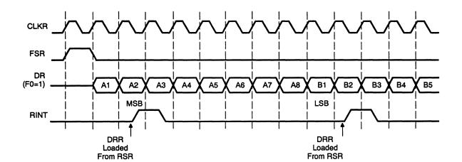
Figure 5-16. Serial Port Receive Continuous Operation
