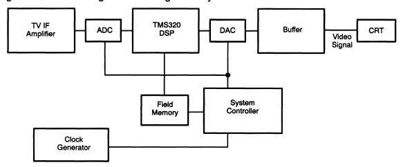
Figure F-13. Video Signal Processing Basic System
