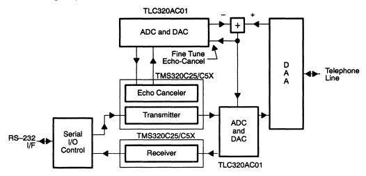
Figure F–11 shows a V.32 bis modem implementation using the C25 and a TLC320AC01. The upper C25 performs echo cancellation and transmit data functions, while the lower C25 performs receive data and timing recovery functions. The echo canceler simulates the telephone channel and generates an estimated echo of the transmit data signal. The TLC320AC01 performs the following functions:
