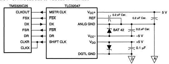
Figure F-3. TMS320C25 to TLC32047 Interface
