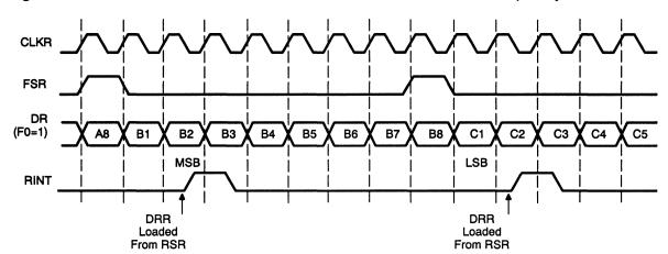
Figure 5-13. Burst-Mode Serial Port Receive at Maximum Packet-Frequency
