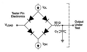
Where:  $I_{OL}$  = 2.0 mA (all outputs)  $I_{OH}$  = 300  $\mu$ A (all outputs)
