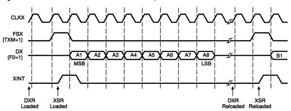
Figure 5-10. Burst-Mode Serial Port Transmit Operation
