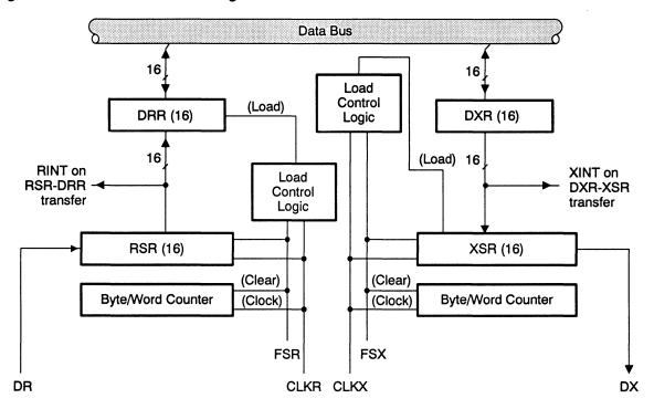
Figure 5-7. Serial Port Block Diagram
