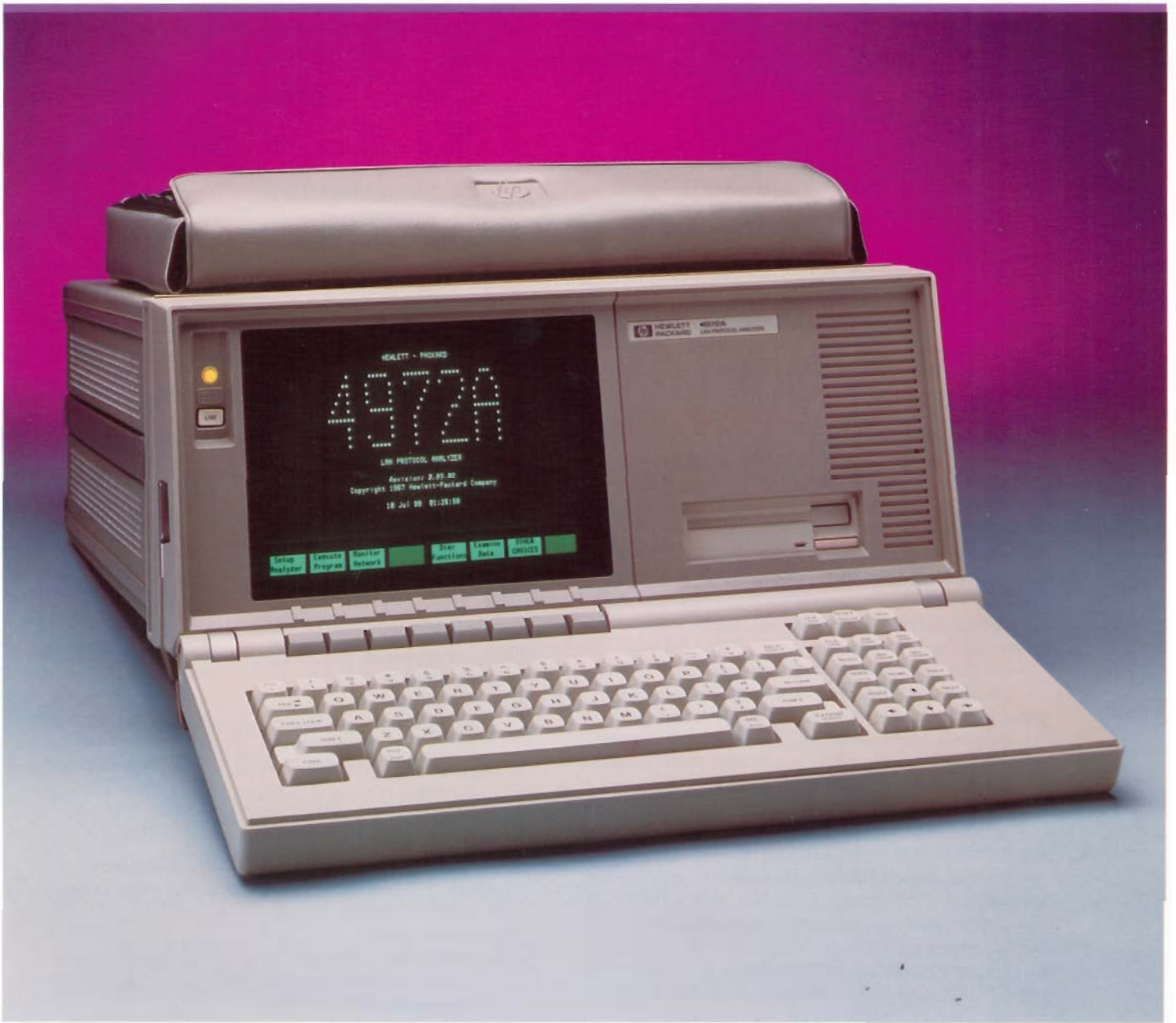
High-resolution display, full-sized keyboard and softkey-driven user interface make the HP 4972A very easy to use.
