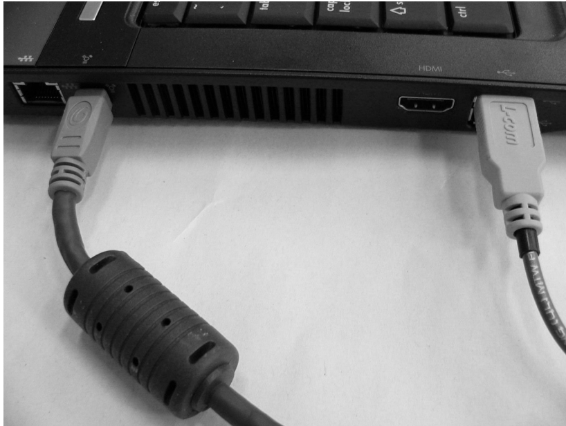
Figure 3-18 IEEE-1394 cable connected to laptop PC (left side of image). EMC grounding cable connected to laptop PC (right side of image).
