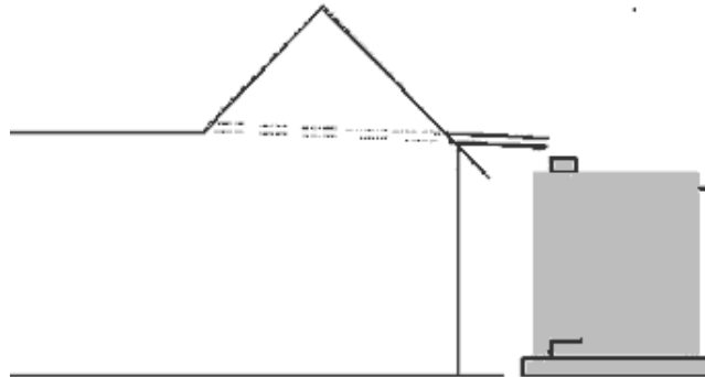
Figure 5 - Pipe has to pass through roof, from central roof courtyard, to tank
