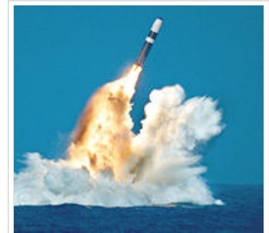
A Trident II SLBM being launched from one of the Royal Navy's 4 Vanguard class submarines as a test launch.
