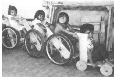
A wood design of the wheelchair, two AHRTAG wheelchairs, and a 'trolley' made from half of a plastic bucket and wood wheels.
