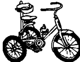
CHILD'S TRICYCLE WITH BODY SUPPORT BOLTED TO FRAME
