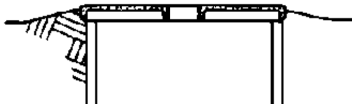
Fig. 7.16. Ferrocement slab (Section)
