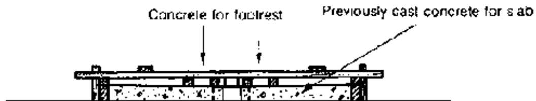
Fig. 7.19. Formwork for the casting of footrests (Section)
