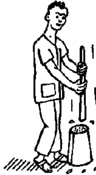
Fig. 7.18. Checking the water content of concrete with a slump cone (A)
