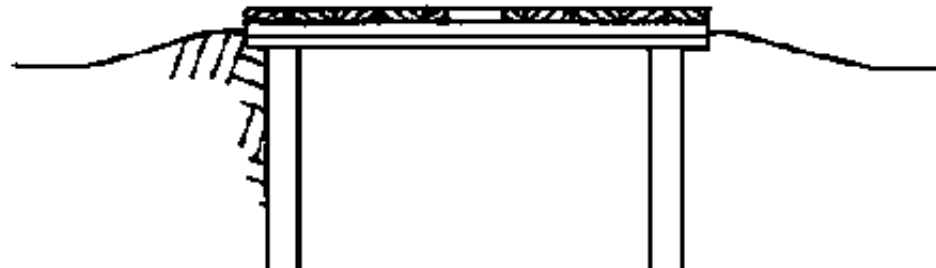
Fig. 7.23. Sawn timber slab (Section)
