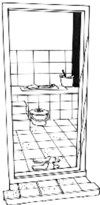
Figure 3.6 The toilet rooms in the Guangxi province eco-san project have a high standard of finish: a prefabricated squatting pan and tiled floors and walls. (Design: Lin Jiang, Nanning, China, 1999).
