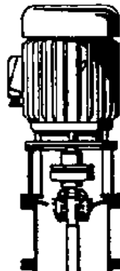
Fig. 21a - Selfpriming centrifugal pump
