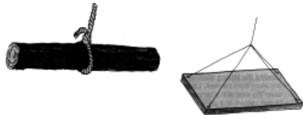
Figure 8-1 - Two Possible Designs for a Bosun’s Chair
