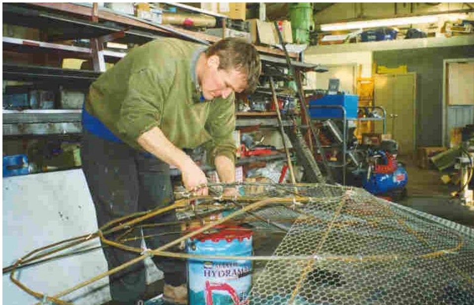
Figure 10. Applying the chicken mesh.
