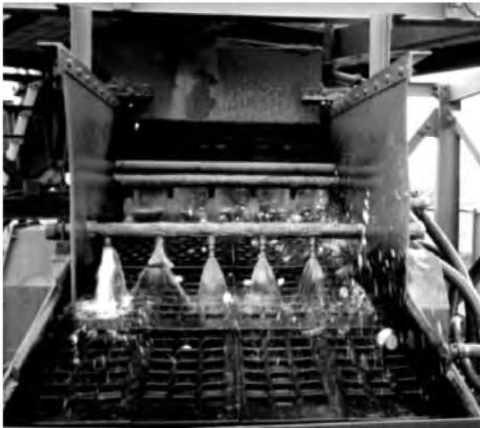
Figure 1.1: Wet screening at Gill Mill Quarry, Oxfordshire
