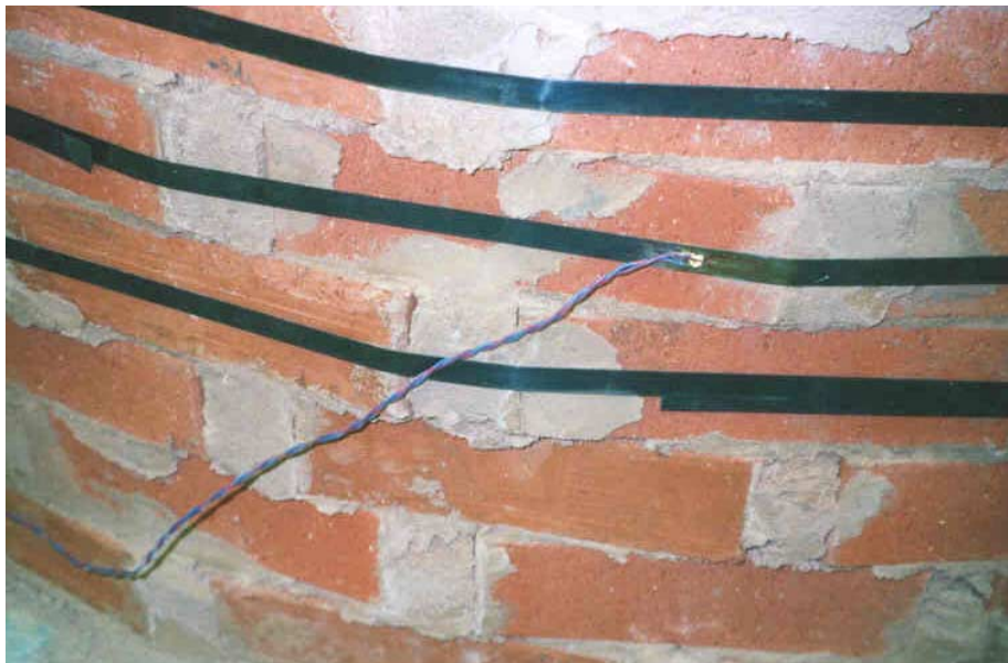
Figure 2 – Strain gauge used to measure hoop stress generated in steel strap during testing.
