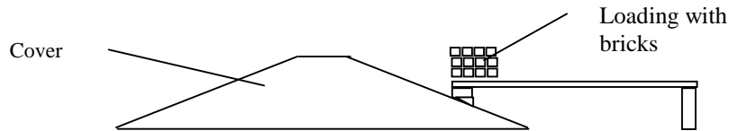
Figure 1 – Loading for point load test
