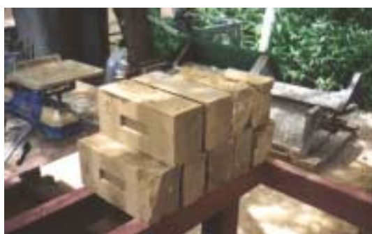
Minor block defects
