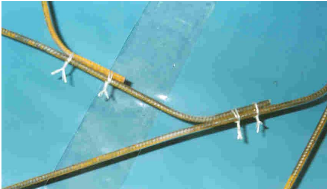
Figure 6. Arrangement for tying spokes to each other.
