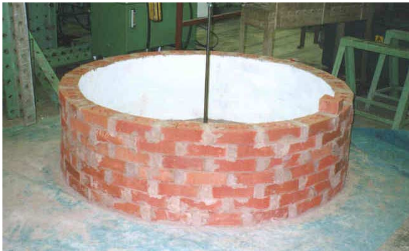
Figure 4 – Brick masonry cylinder specimen
