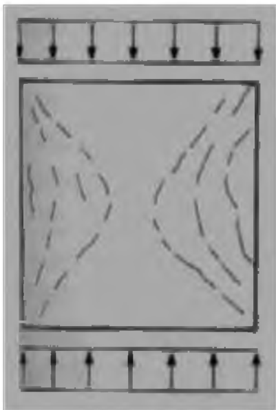
Figure 5.2a: Cracking Pattern Of a Cube
