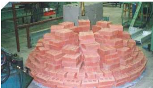
Figure 21 - Tank cover loaded to 1000kg
