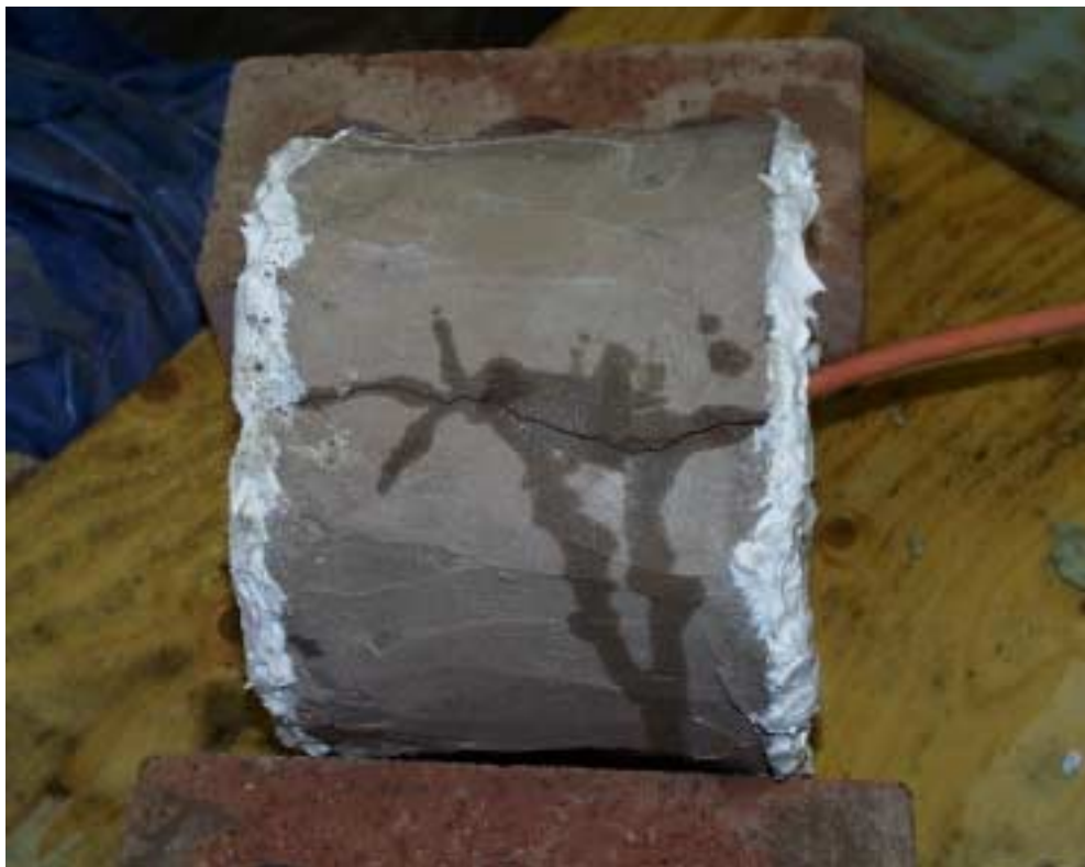
Figure 22: Leakage through a crack
