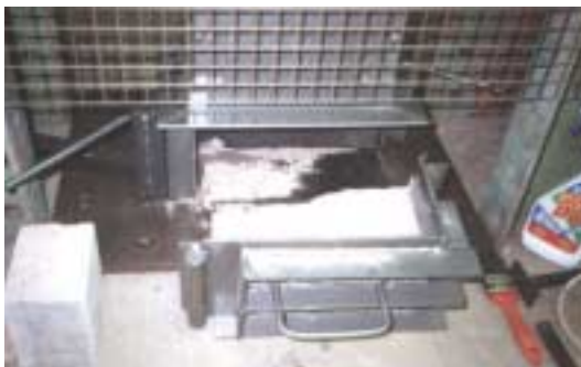
Two part mould in use, illustrating the problem with block ejection
