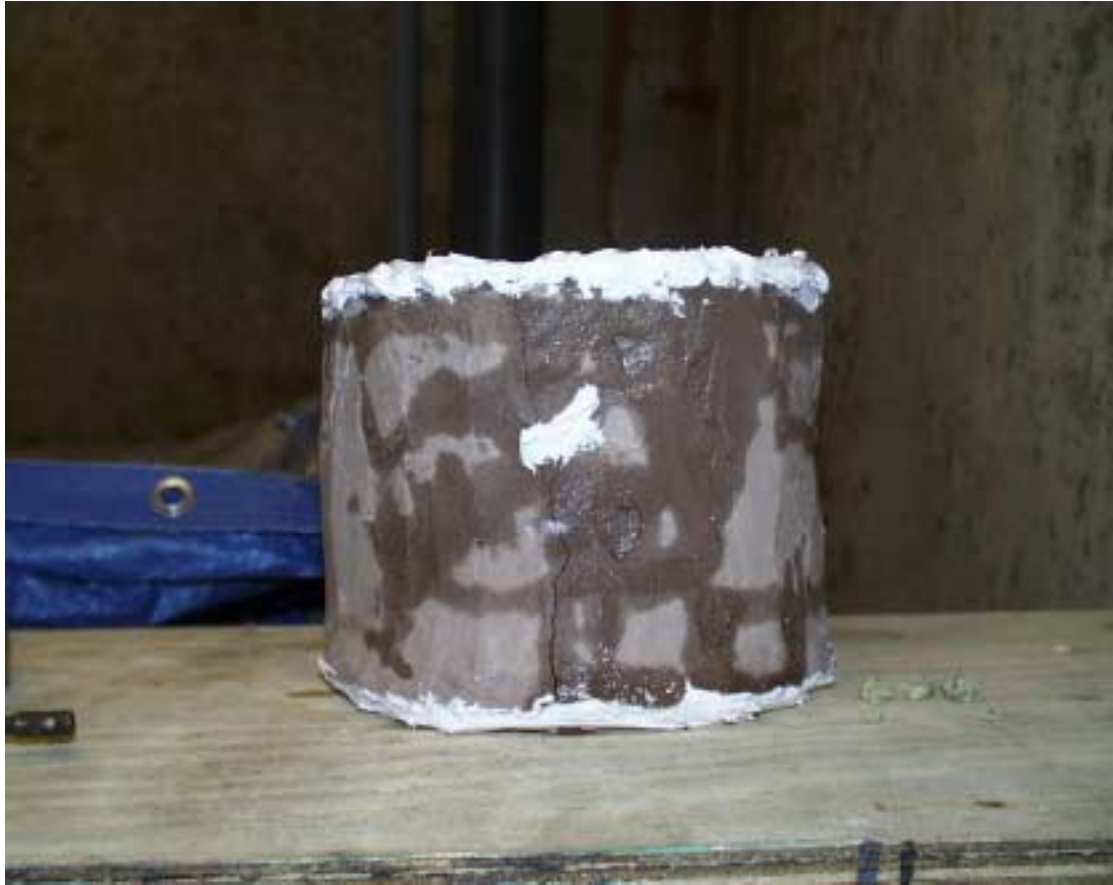
Figure 23: A sample with end leakage
