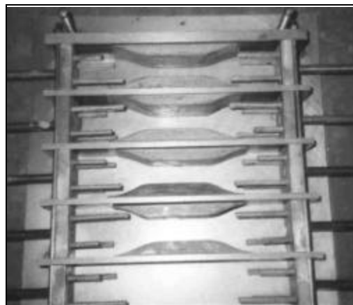
Fig. 5.3 moulds used to cast samples
