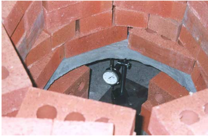
Figure 3 – dial gauge in place to test deflection of cover under load
