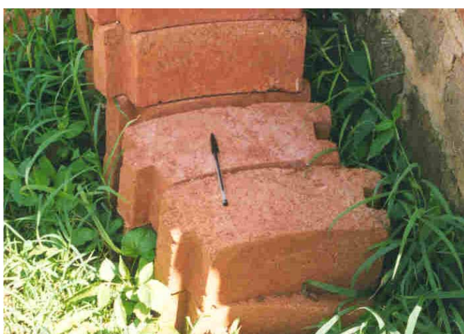
(Figure 6.3 – Curved blocks after curing)
