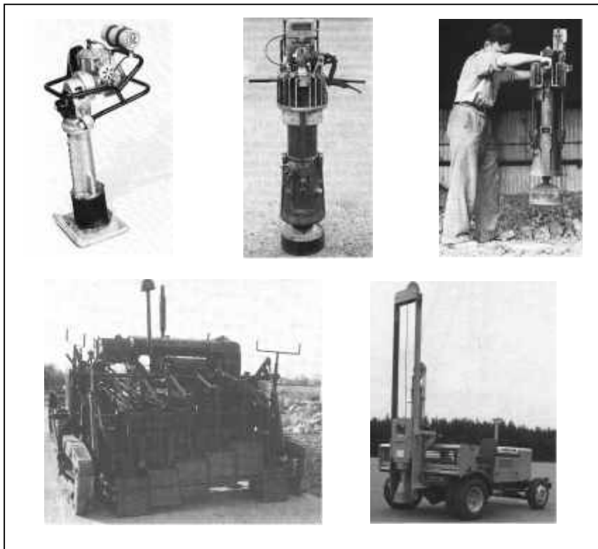
Figure 2.16 – Civil engineering compaction equipment using impact
