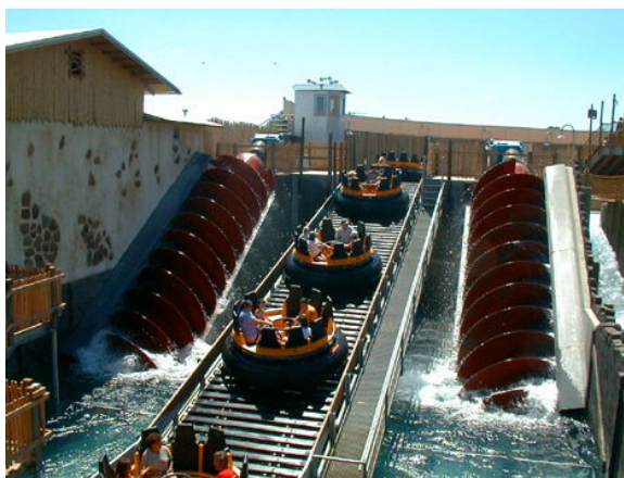
Fig. 5 Archimedian Screws installed in a theme park (29)
