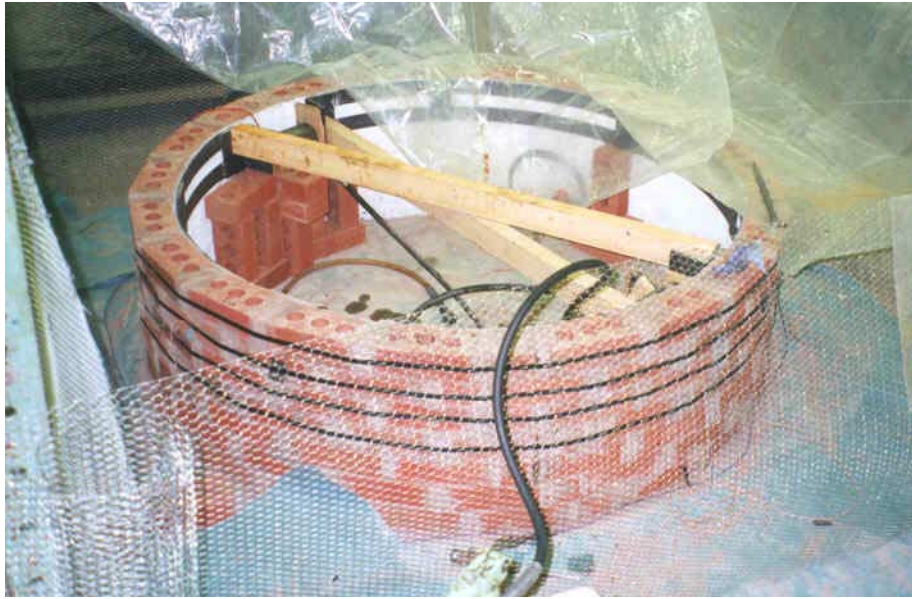
Figure 1 – Tests arrangement for externally reinforced brick cylinders
