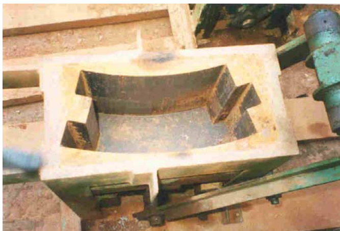
(Figure 6.2 – Mould for producing curved blocks)
