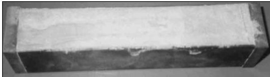
Figure 5.15 Micro crack development in restrained sample
