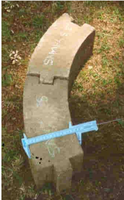
Figure 11 – Showing the interlocking blocks used for the tanks
