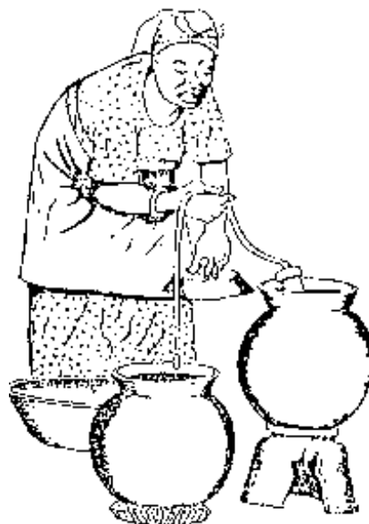
Fig. 18: Siphon filter. Filtration is started by sucking the water by mouth into the siphon system
