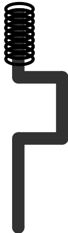
Figure 2: using bent steel rod to rotate drill.
