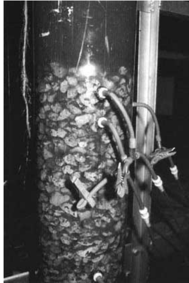
Photo 7 Vertical Roughing Filter Column
