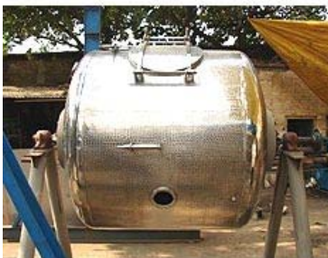
Figure 4: Large butter churn. Photo: Courtesy of Jaya Industries.
