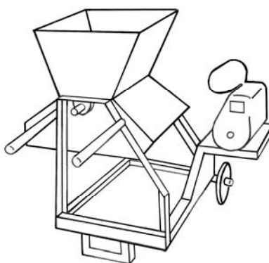
Figure 3: A cassava chipper Illustration: Neil Noble/Practical Action
