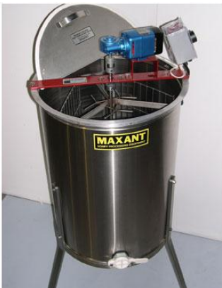
Figure 2: Nine-frame electric honey extractor. Photo courtesy of Mazant Honey Processing Equipment.
