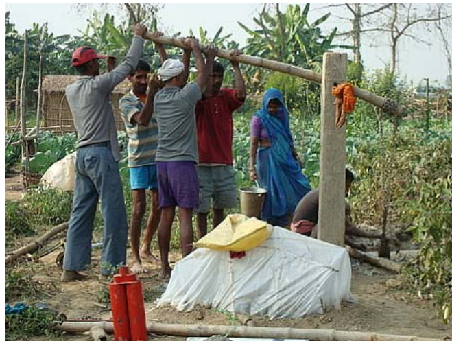
Figure 6: Farmers, from Mainhiya Village Development Committee, installing a treadle pump for irrigation. Video: Practical Action Nepal.
