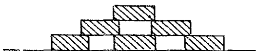
FIGURE 3. STACK THE BARS SO THAT AIR CAN CIRCULATE AROUND AND THROUGH THEM
