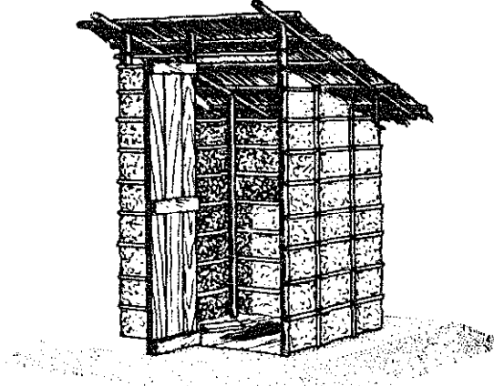
WATTLE HOUSE WITH PALM THATCH ROOF
