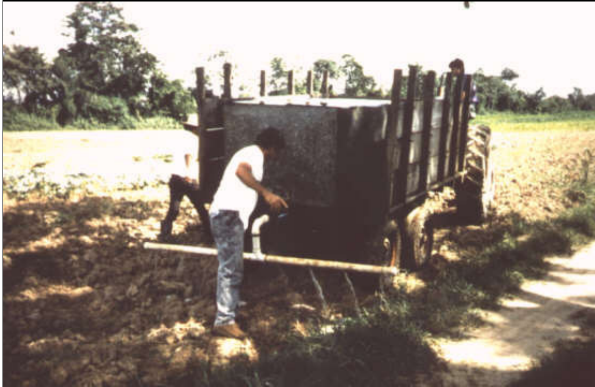
Device for slurry distribution by tractor.
