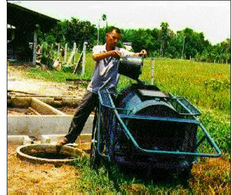
Drying of digested sludge and sludge disposal in Thailand
