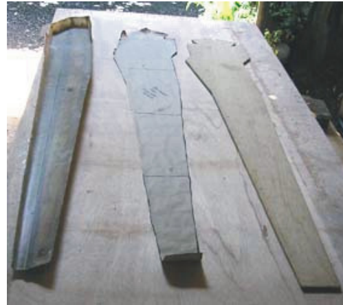
BACKWARD MOULD PAPER TEMPLATE PLYWOOD TEMPLATE
