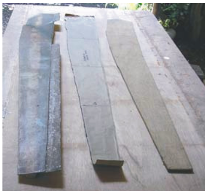
WINDWARD MOULD PAPER TEMPLATE PLYWOOD TEMPLATE
