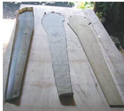
BACKWARD MOULD PAPER TEMPLATE PLYWOOD TEMPLATE
