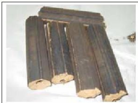
Pic. 4: Extruder briquettes from Thai Production /5/
