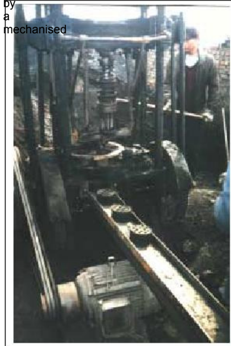
Pic. 8: Chinese semi-mechanised briquetting press /7/
