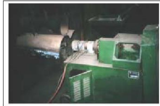
Pic. 3: Locally manufactured screw extruder from Mali /2/
