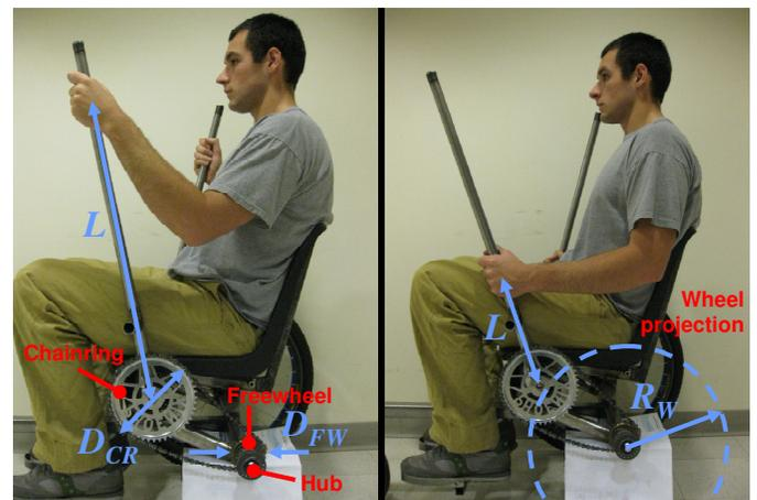
a. LFC in low gear | b. LFC in high gear
