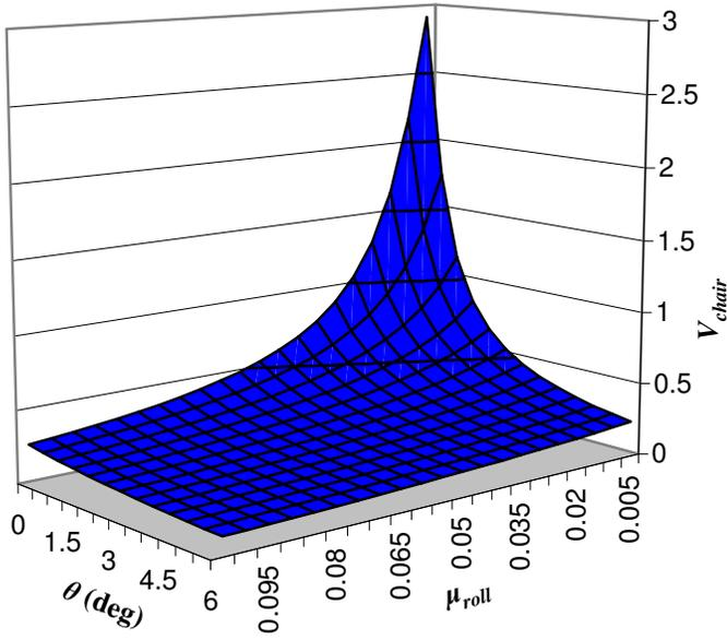
Figure 5. Attainable velocity at peak efficiency power output
