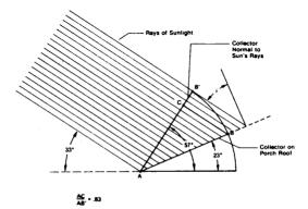
Sunlight intercepted by a solar collector in two orientations. In position AB it intercepts only a fraction (AC/AB') as much solar energy as it does when it is perpendicular to the sun's rays, as in position AB'. The angle between the rays of sunlight and a line perpendicular to the collector, labelled in the figure, is called the angle of incidence.
