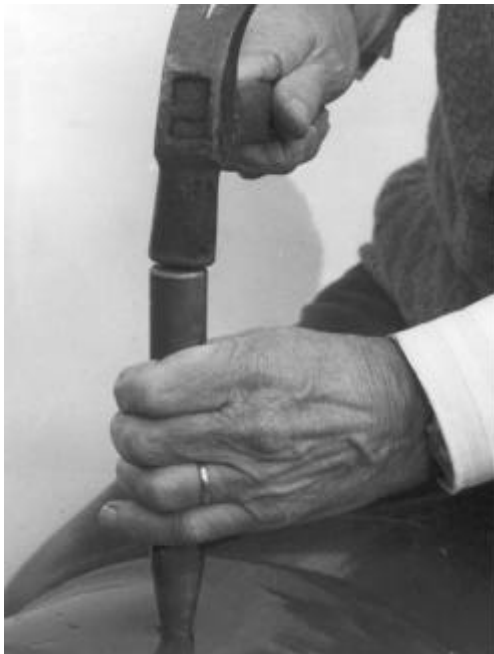
Photo 3: By using the steel cone and hammer widen one hole until a 1/2" piece of pipe fits in.
