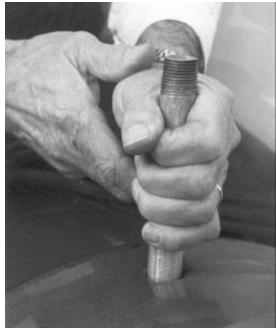
Photo 4: The thread-end of the pipe must be kept outside of the drum. All pipes stand perpendicular of the drum.
