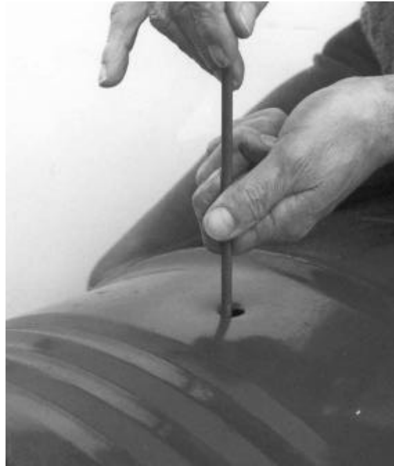
Photo 2: Deburr the holes with a round file until the holes have diameter of 18 mm.
