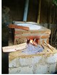
fig 1b: Patsari improved cookstove made of bricks and mortar and ruble filling
