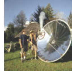
Solar Satellite Cooker: The parabolic shape focuses the sunlight on a single point
