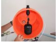
Fig 1: Float valve inside the external holding bucket
