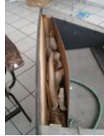
Fig 3: Sawdust may be a decent insulator but it's very messy when uncontrolled. Also encountered were styrofoam peanuts, and various loose ceramic tiles. *Materials
