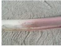
Fig 6: Melted collection trough, with glue.
