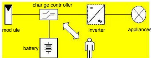
Figure 2: Block diagram of a PV system
