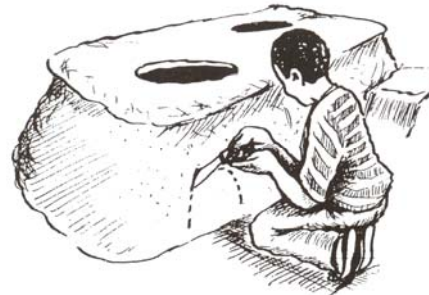
Figure 5.31 Cutting out the door
