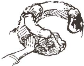
Figure 5.102 Putting mud around the three stones
