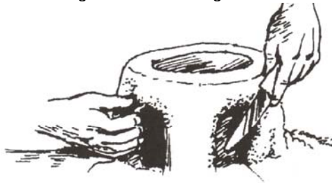
Figure 5.15 Cutting out the doors
