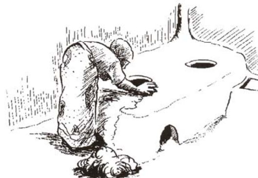
Figure A2.5 Filling in the crack
