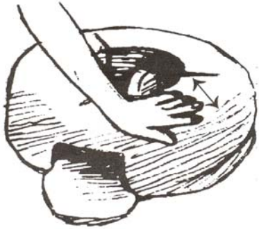
Figure 3.5 Measuring the wall thickness
