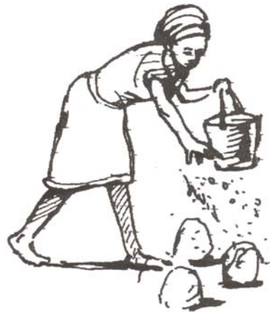
Figure 5.96 Sprinkling water on the stones
