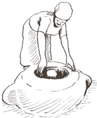
Figure 5.64 Smoothing out the stove
