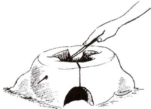
Figure 5.68 Making a smoke vent
