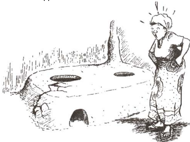
Figure 7.3 Let the stove dry for at least two weeks before use to avoid cracks
