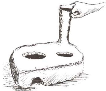
Figure 3.15 Ensuring the chimney diameter is correct
