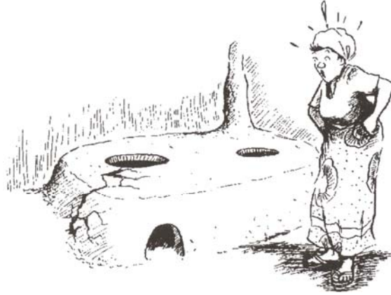
Figure A2.1 Cracks may appear on stoves after prolonged use
