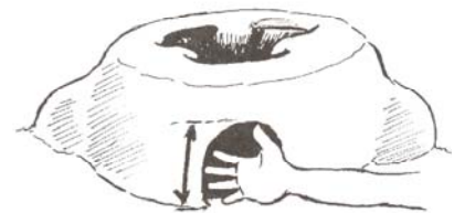
Figure 5.66 The height of the stove door
