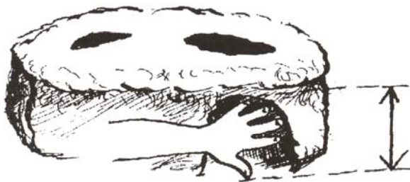
Figure 5.70 Height of the stove door
