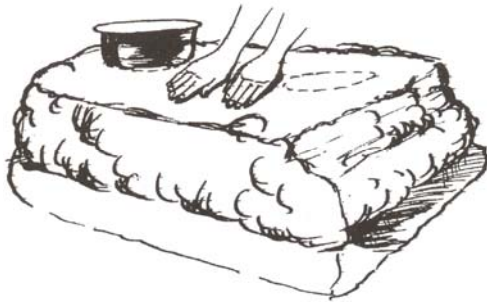
Figure 5.28 Marking the Pot-holes position
