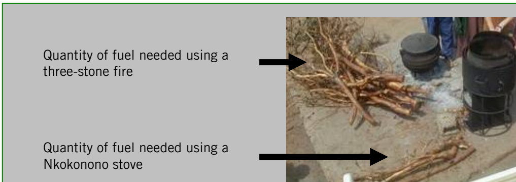
Figure 3: The use of an improved institutional stove can appreciably reduce fuel consumption (photo: Peter Scott)
