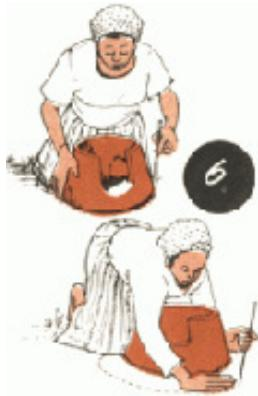
***Measure a space of at least two flat hands away from the wall, check that the liner is still wet, and place it wide side down on the floor outside that space.***
