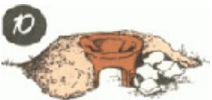
***Your jiko liner is in place now, so don't lean on it. Add the rounded stones. Its very simple. First add the stones, then fill the gaps with the prepared soil mix and put on a thick layer of prepared soil.***
