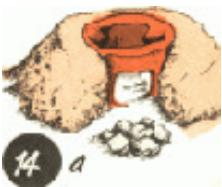
***Flatten the grate both inside and outside. And put down more wet flat stones a hand's length away from the fire opening and a thumb's distance away from the stove sides.***
