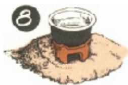
***To make sure your cooking sufurias will stand straight on the jiko, put a sufuria on the liner just as if you were going to cook with it, and pour in some clean water. Push the liner into the foundation until the water in the sufuria is level.***
